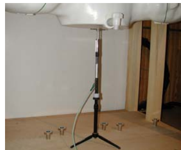
Figure 12.1 Dipole Validation Test Setup
