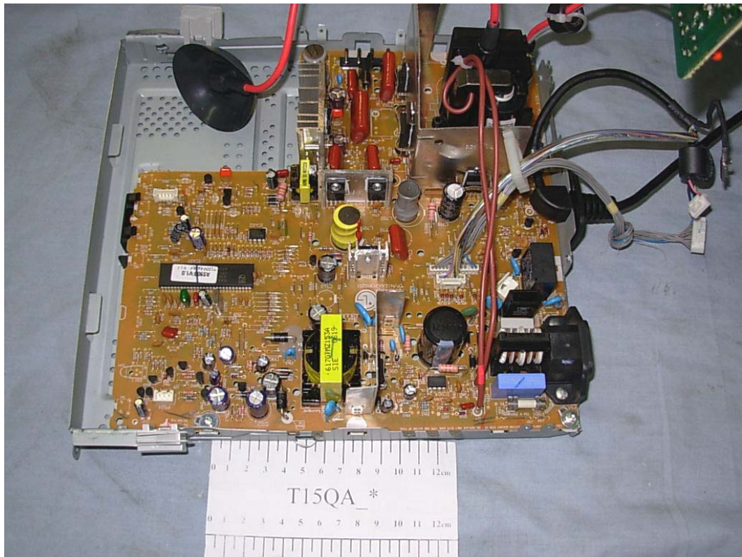
FIGURE 8 CRT MONITOR (M/N: T15QA-*) MAIN BOARD 1 (COMPONENT SIDE)
