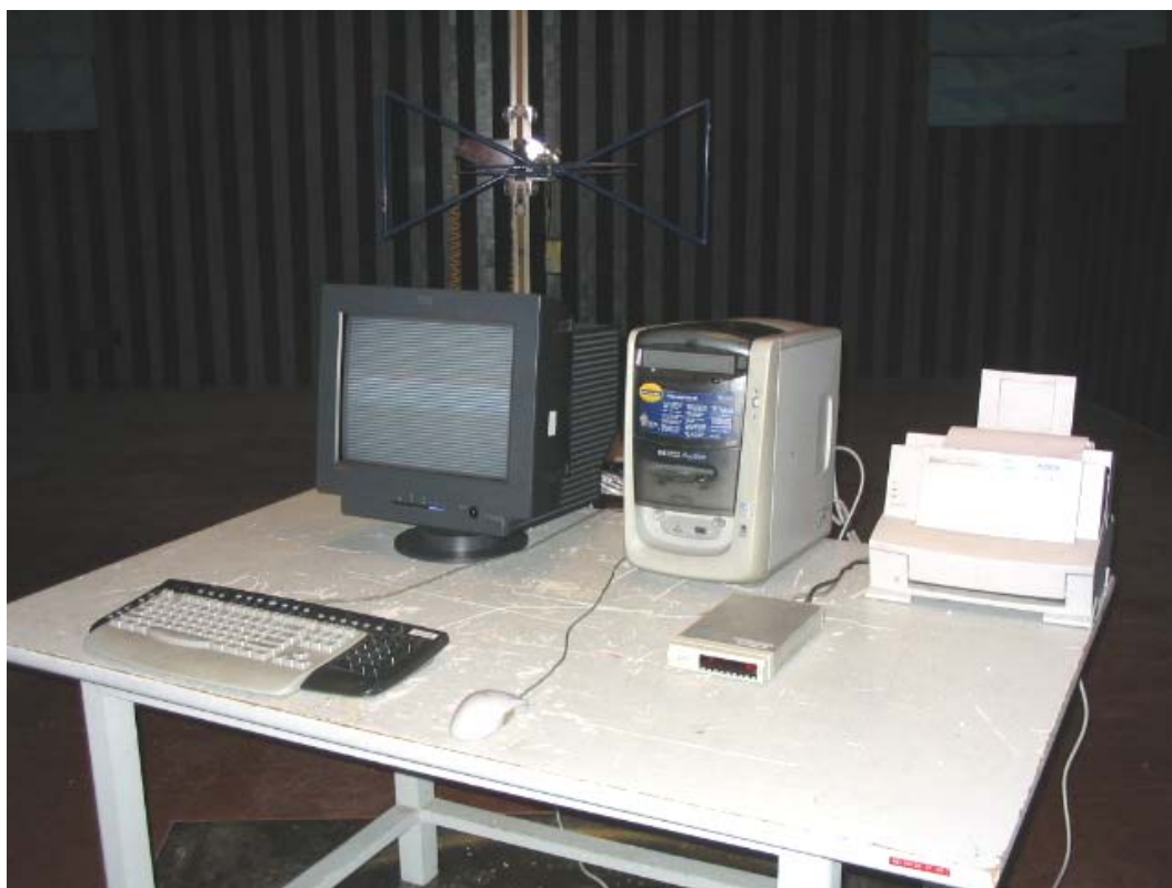
SETUP WITH MAXIMUM DETECTED EMISSION AT HORIZONTAL POLARIZATION (M/N: 6737-*6* /A)
