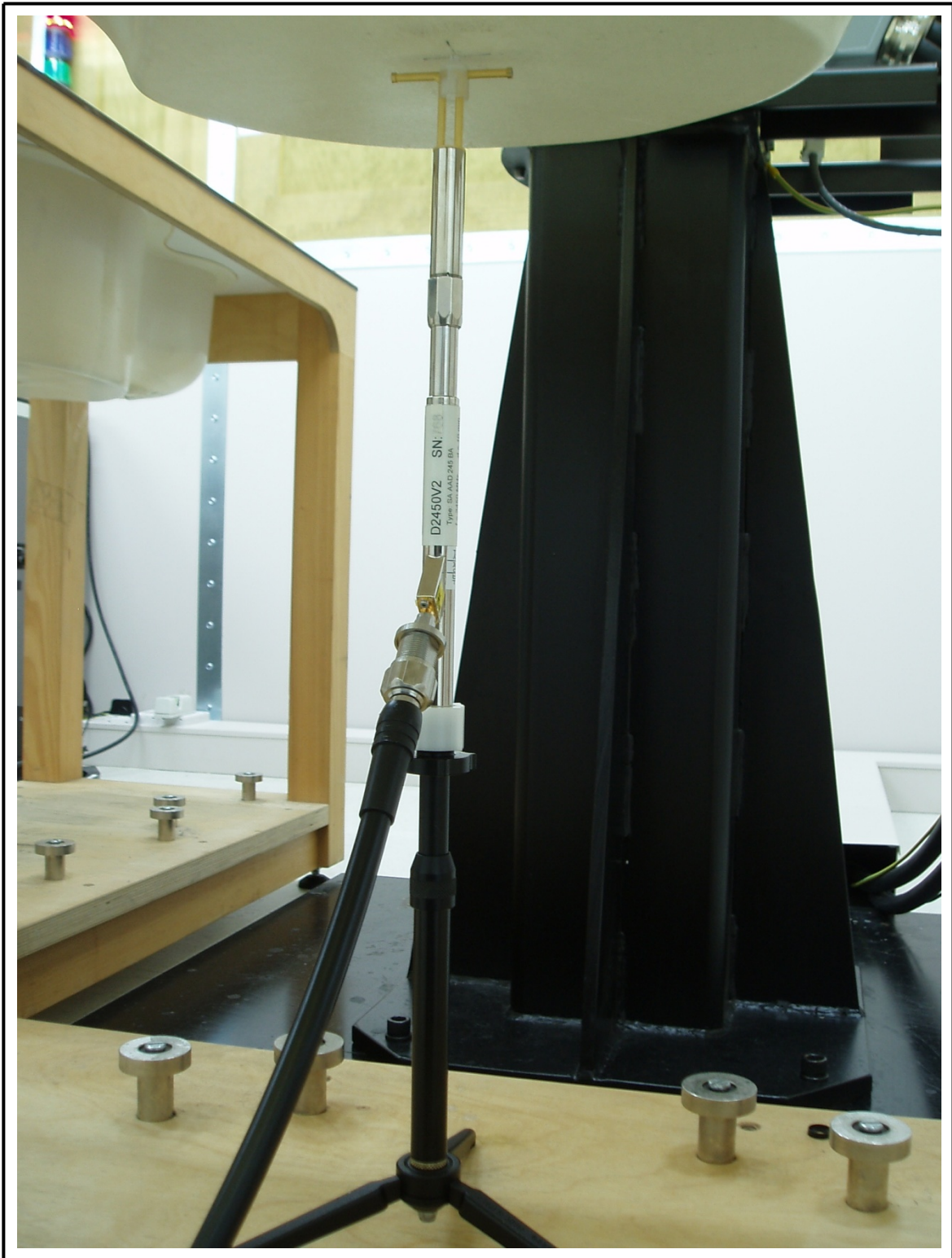
Figure 3 2450 MHz Dipole Validation Test Setup
