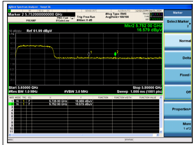
High channel Band edge (Peak) - Band 2C
