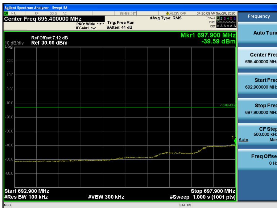
LTE Band 12 / 1.4 MHz / QPSK - RB Size/Offset (6/0)
