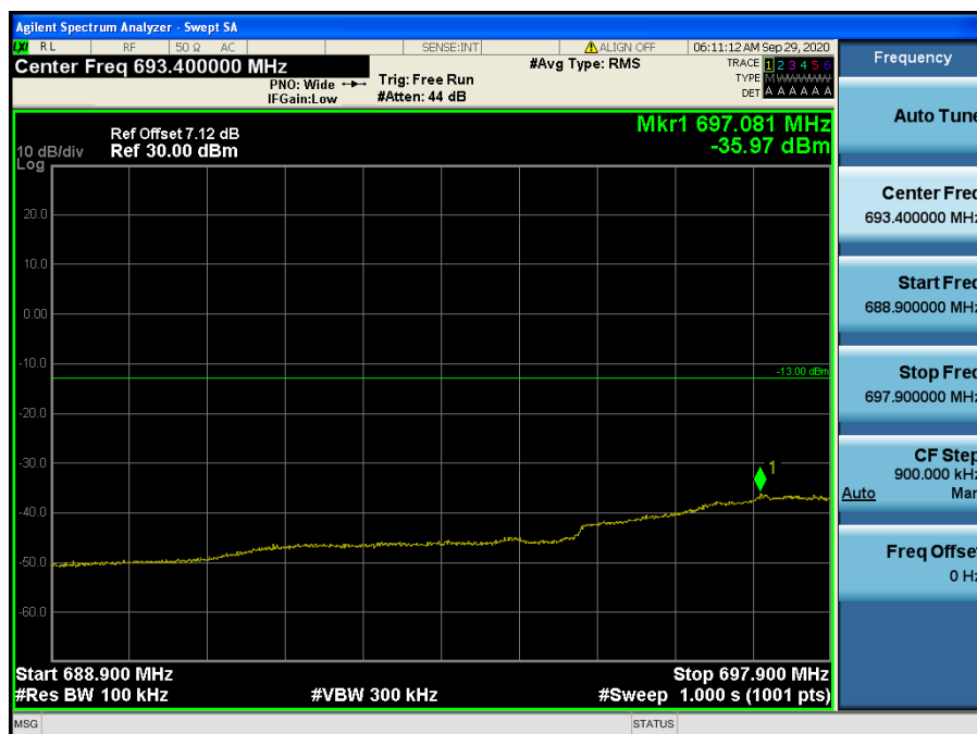
LTE Band 12 / 10 MHz / QPSK - RB Size/Offset (25/0)
