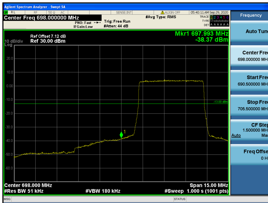
LTE Band 12 / 5 MHz / QPSK - RB Size/Offset (25/0)
