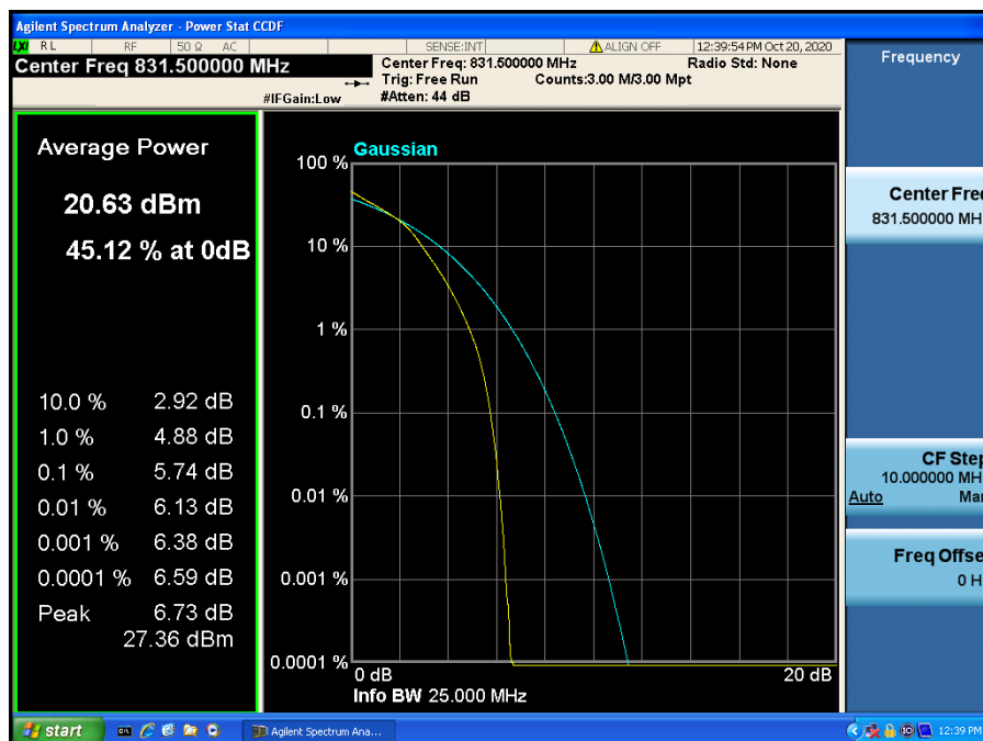
LTE Band 26 / 15 MHz / 16QAM - RB Size 75
