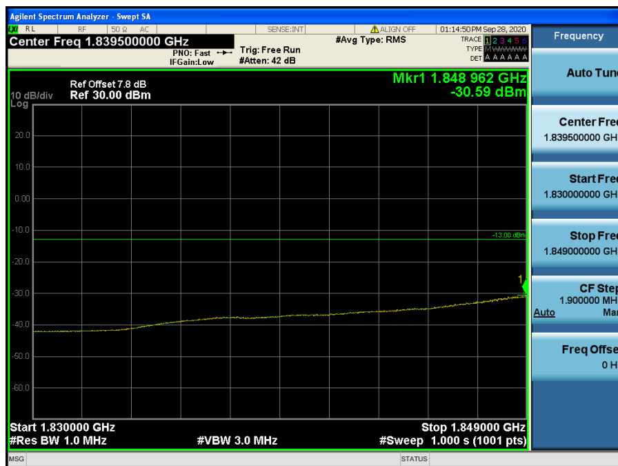
LTE Band 2 / 20 MHz / QPSK - RB Size/Offset (50/0)
