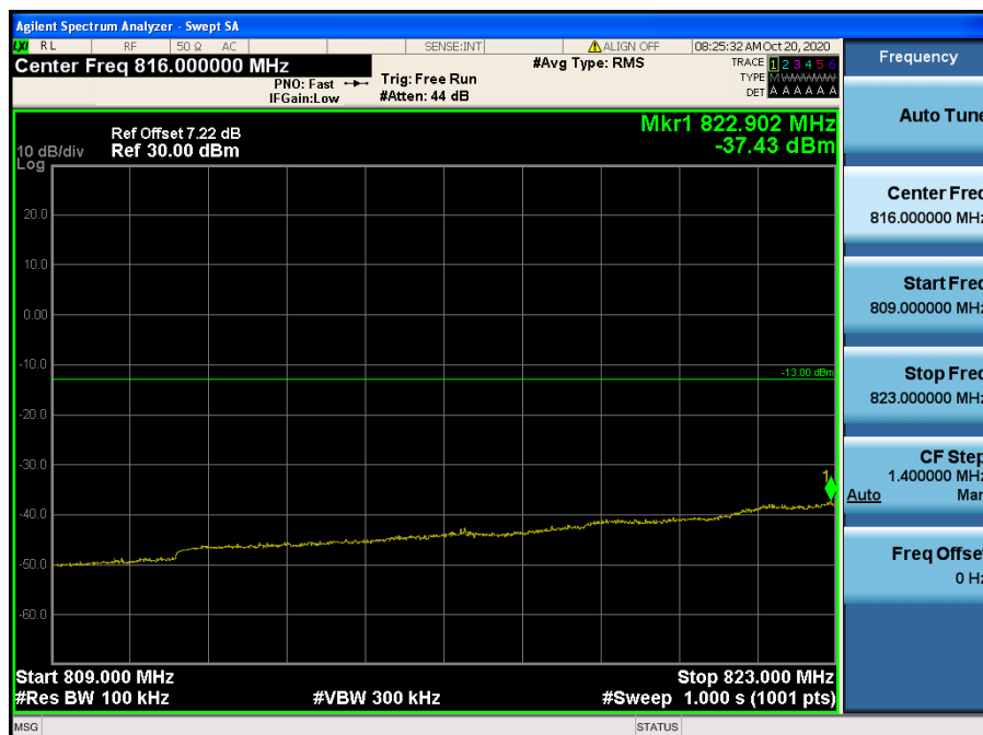
LTE Band 26 / 15 MHz / QPSK - RB Size/Offset (75/0)
