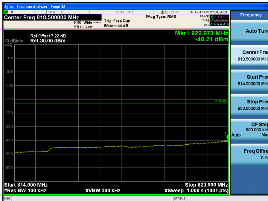
LTE Band 26 / 10 MHz / QPSK - RB Size/Offset (50/0)
