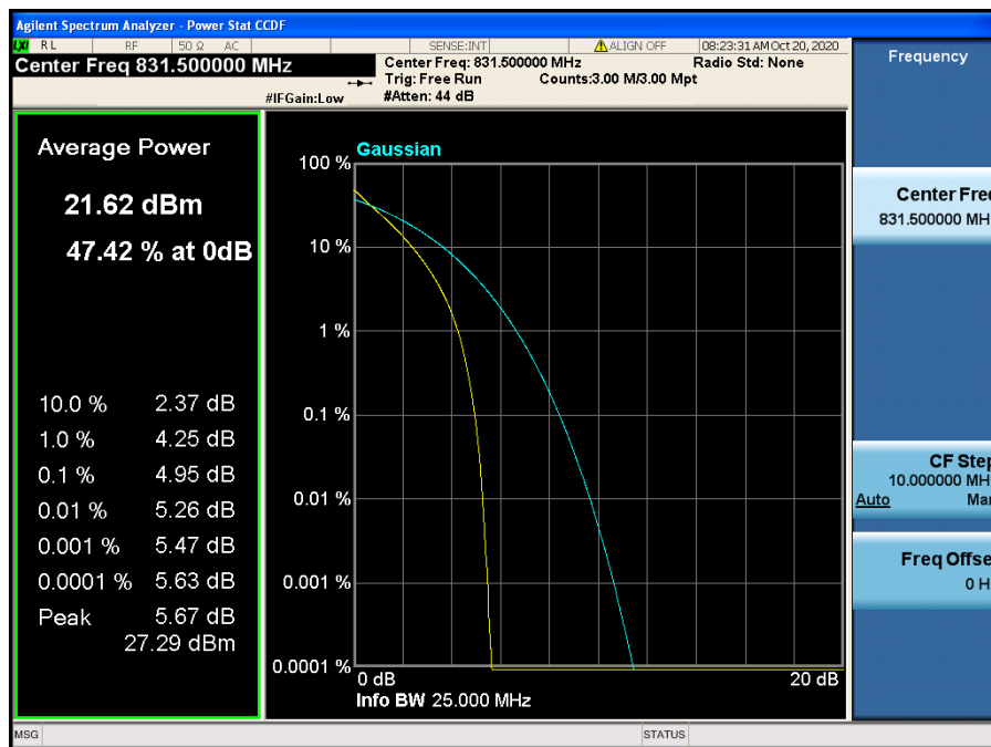
LTE Band 26 / 15 MHz / QPSK - RB Size 75
