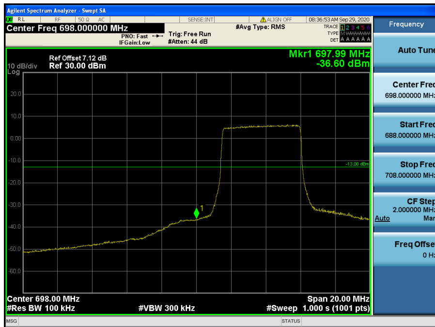
LTE Band 12 / 10 MHz / 16QAM - RB Size/Offset (25/0)
