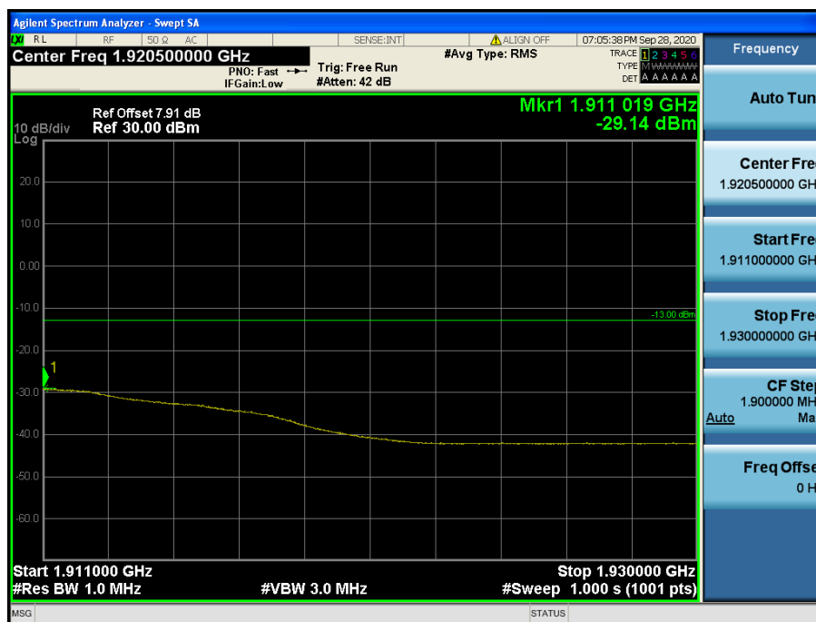
LTE Band 2 / 20 MHz / 16QAM - RB Size/Offset (50/50)
