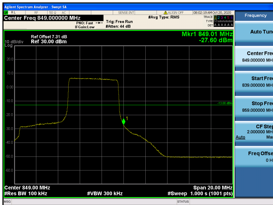
LTE Band 26 / 10 MHz / QPSK - RB Size/Offset (25/25)
