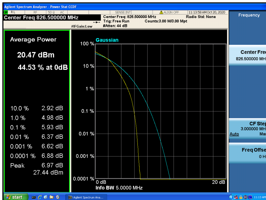
LTE Band 26 / 5 MHz / 16QAM - RB Size 25
