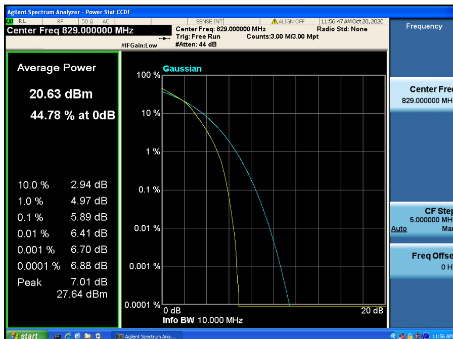
LTE Band 26 / 10 MHz / 16QAM - RB Size 50
