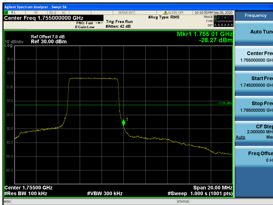
LTE Band 4 / 10 MHz / QPSK - RB Size/Offset (25/25)
