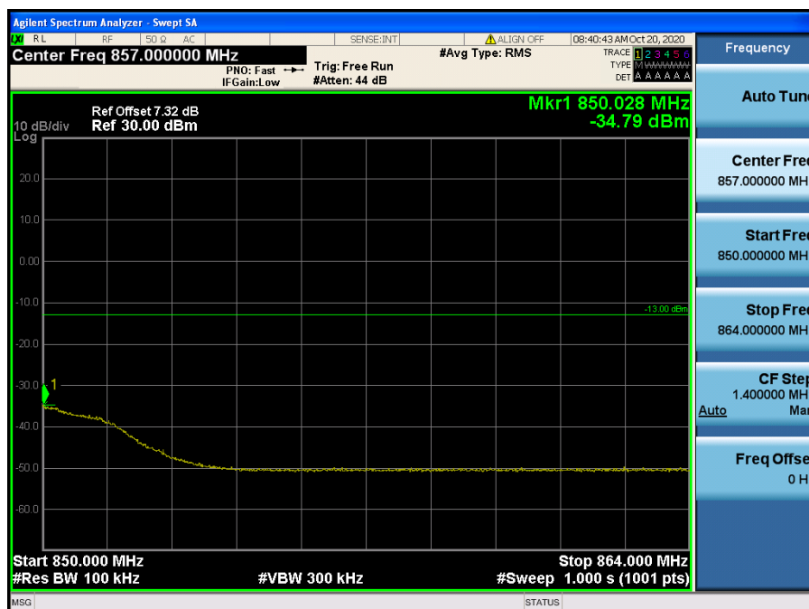
LTE Band 26 / 15 MHz / QPSK - RB Size/Offset (36/39)
