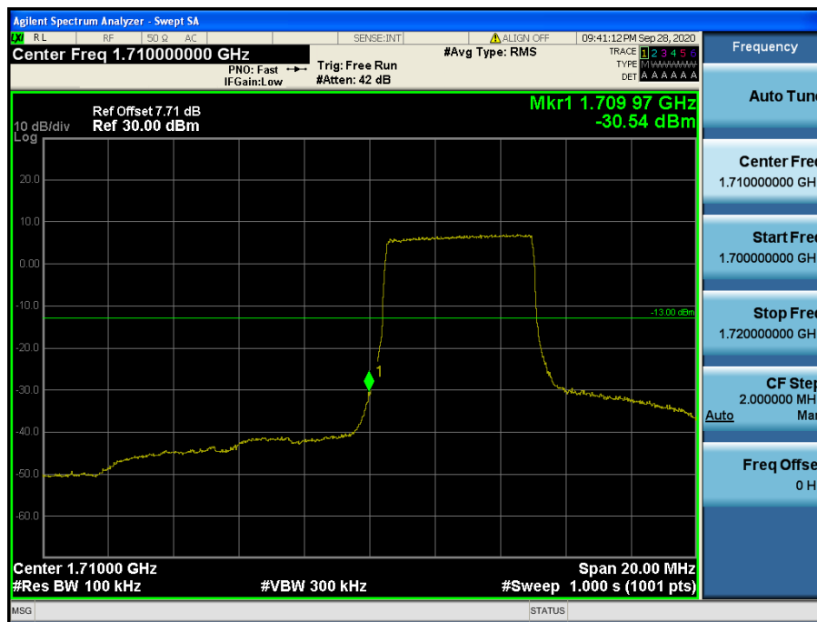
LTE Band 4 / 10 MHz / QPSK - RB Size/Offset (25/0)
