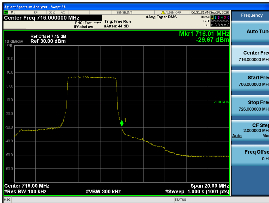
LTE Band 12 / 10 MHz / QPSK - RB Size/Offset (25/25)
