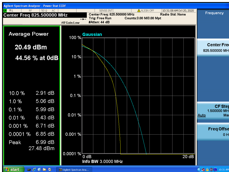
LTE Band 26 / 3 MHz / 16QAM - RB Size 15
