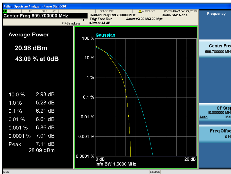
LTE Band 12 / 1.4 MHz / 16QAM - RB Size 6
