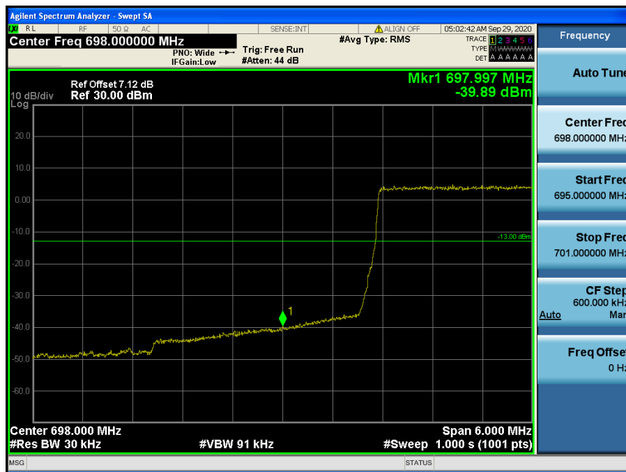
LTE Band 12 / 3 MHz / QPSK - RB Size/Offset (15/0)
