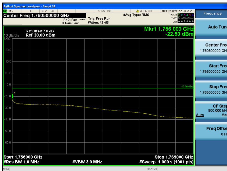
LTE Band 4 / 10 MHz / QPSK - RB Size/Offset (25/25)
