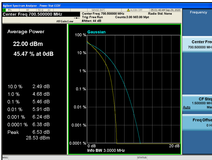
LTE Band 12 / 3 MHz / QPSK - RB Size 15
