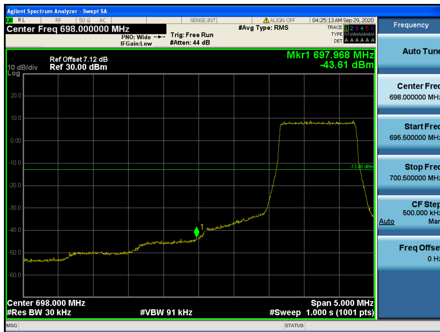
LTE Band 12 / 1.4 MHz / QPSK - RB Size/Offset (6/0)
