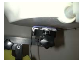
Figure 14.11 Body SAR Test Setup -- w/o Holster --
