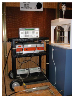
Figure A.0 Dipole Validation Test Setup
