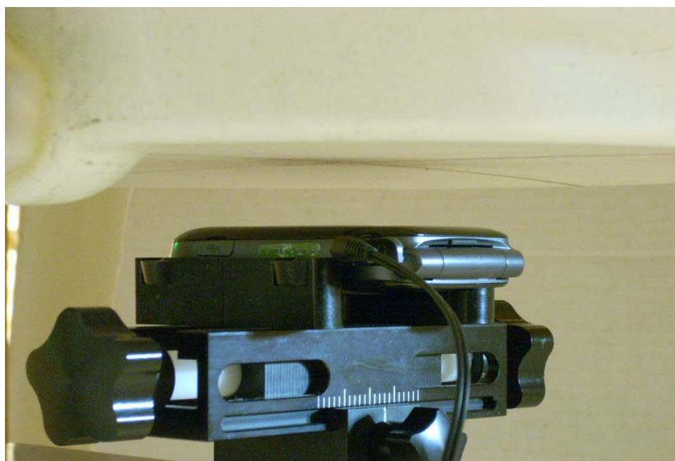
Figure 19-6 SAR Test Setup Photo 6 – Back at 2.0 cm
