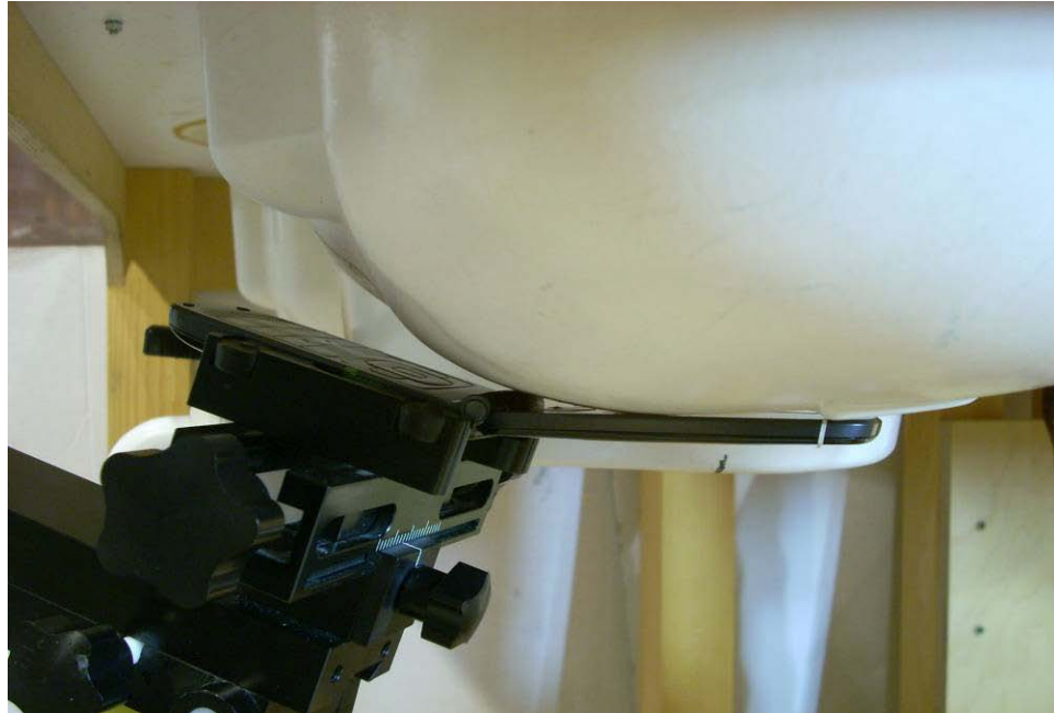
Figure 19-3 SAR Test Setup Photo 3 – Left Touch
