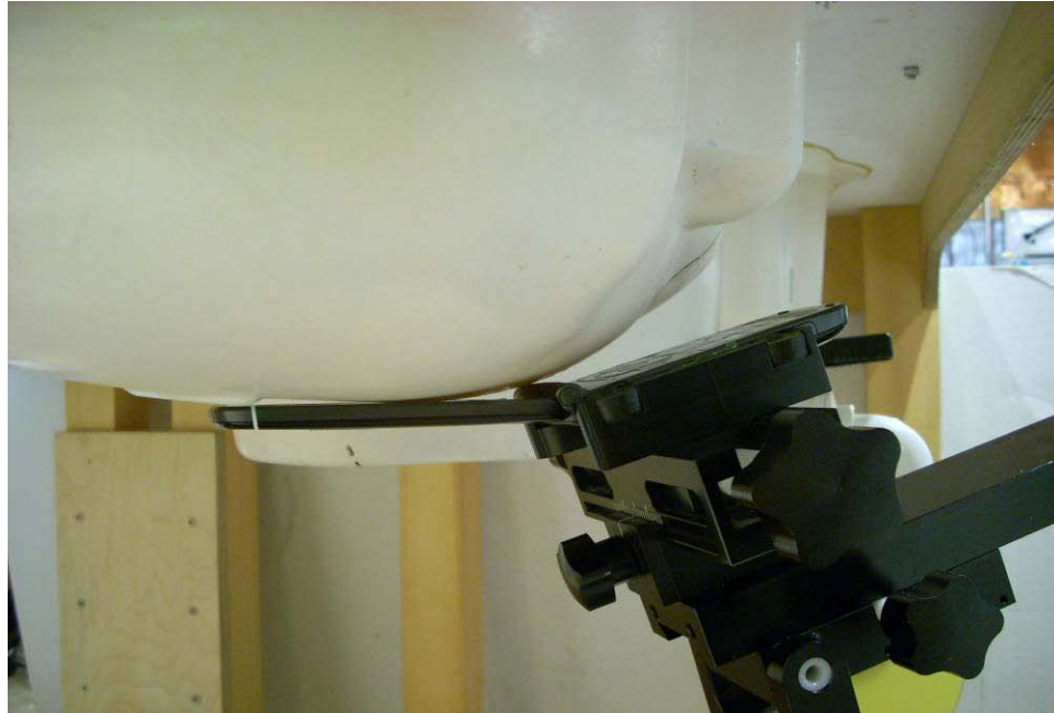
Figure 19-1 SAR Test Setup Photo 1 – Right Touch
