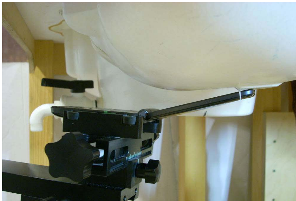
Figure 19-4 SAR Test Setup Photo 4 – Left Tilt
