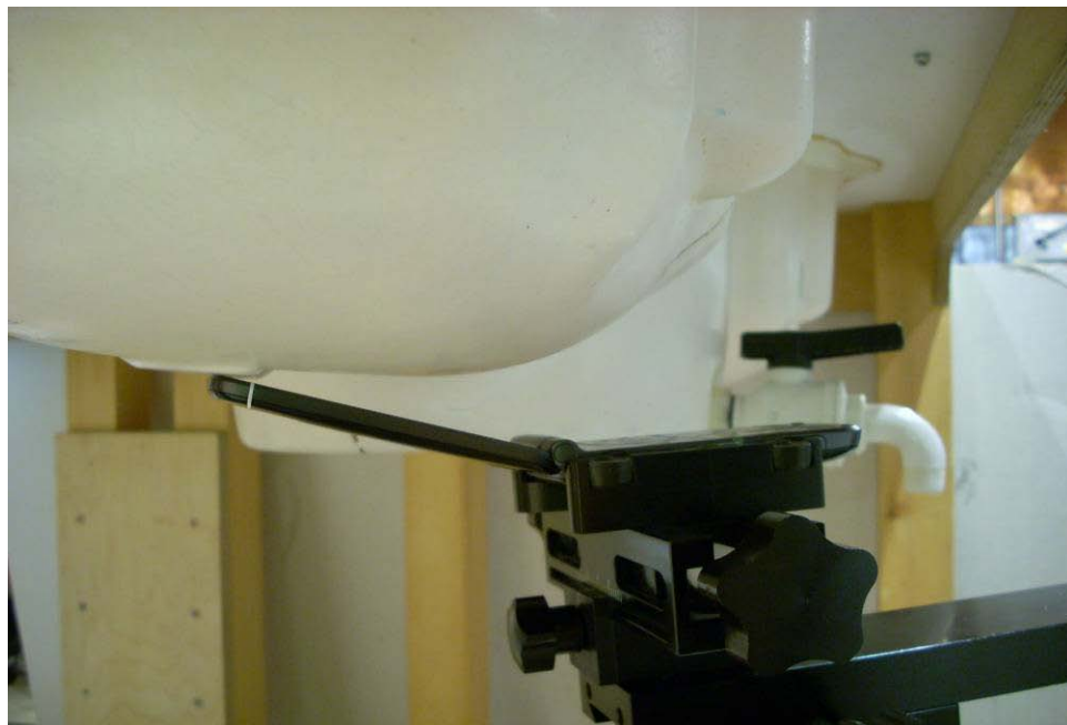
Figure 19-2 SAR Test Setup Photo 2 – Right Tilt
