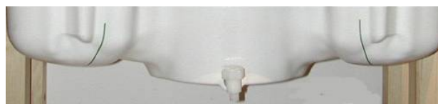
Figure 7-2 SAM Twin Phantom Shell
