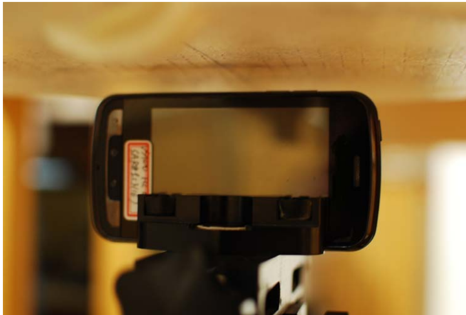
SAR Test Setup Photo 10: Left at 1.0 cm
