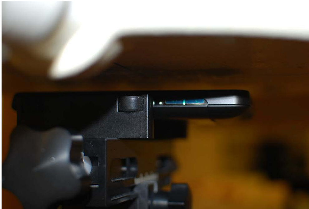
Figure 22-6 SAR Test Setup Photo 7: Front Side
