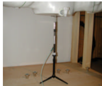
Figure 12.1 Dipole Validation Test Setup
