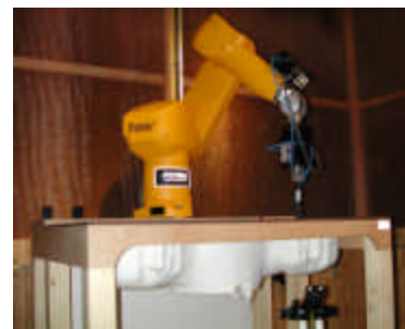
Figure 6.1 DASY4 Test System
