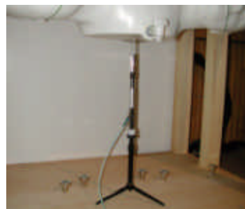
Figure 12.1 Dipole Validation Test Setup
