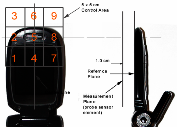
Figure 13 E/H-Field Emissions Test Setup Diagram
