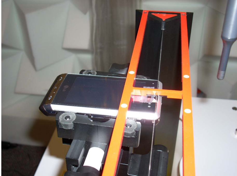
Figure 17-1 Ear Reference Point HAC Phantom Alignment
