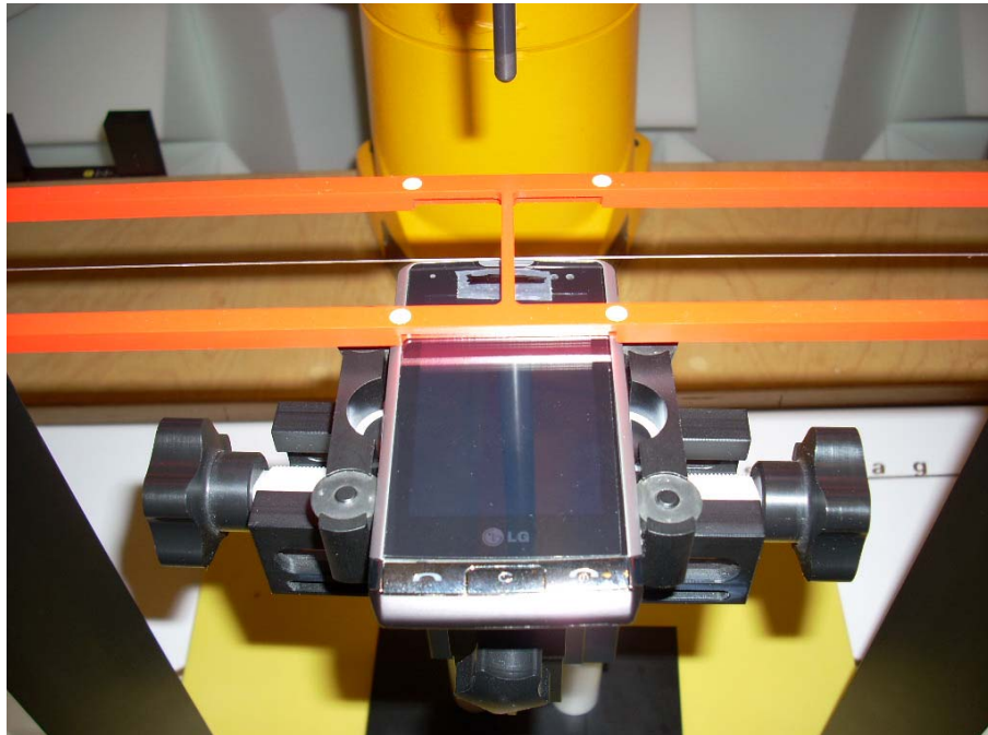
Figure 17-2 HAC Phantom Plane Alignment
