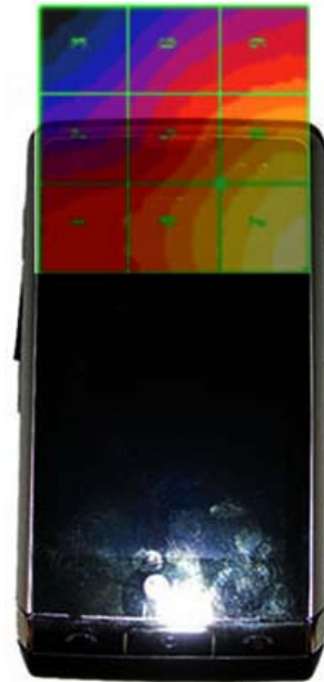
Figure 17-5 H-Field WD Scan overlay
