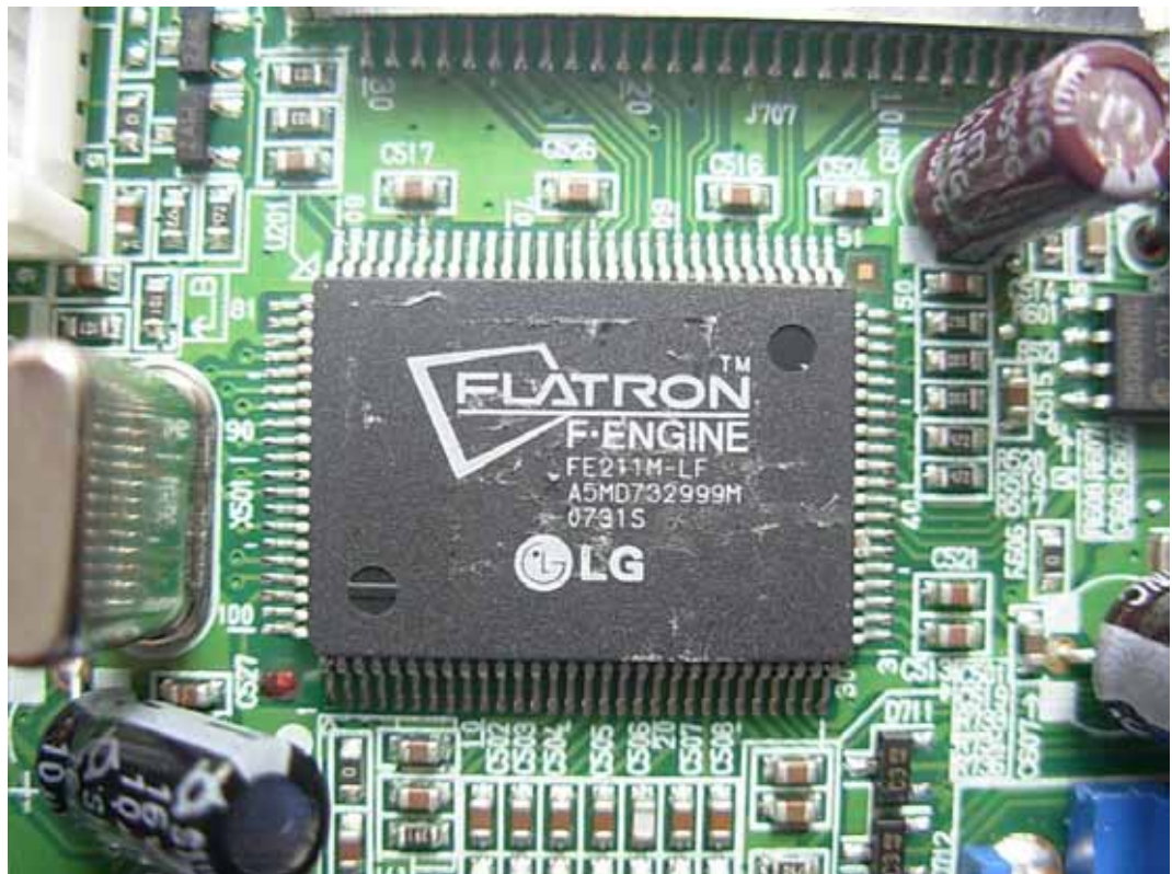
FIGURE 9 LCD MONITOR (M/N: W1642ST) CHIP ON MAIN BOARD
