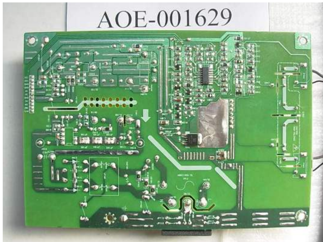
FIGURE 11 LCD MONITOR (M/N: W1752TT) POWER BOARD (SOLDERED SIDE)
