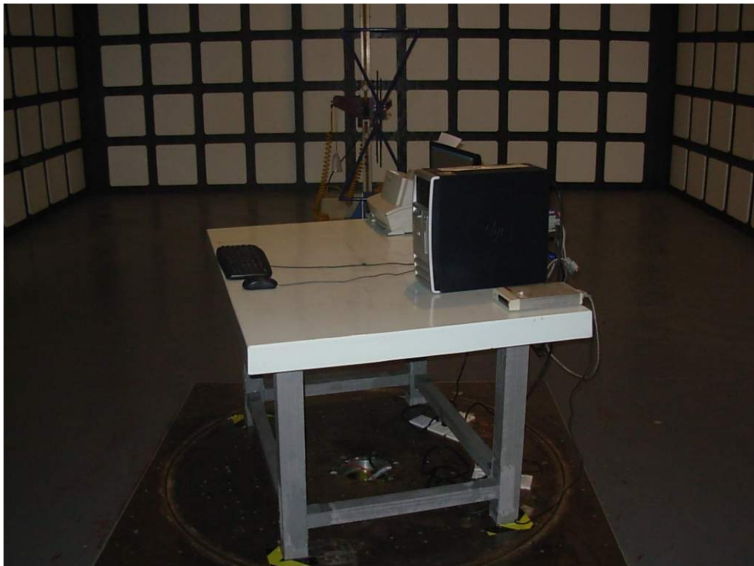
SETUP WITH MAXIMUM DETECTED EMISSION AT VERTICAL POLARIZATION (VGA 1440*900@60Hz, BELOW 1GHz)
