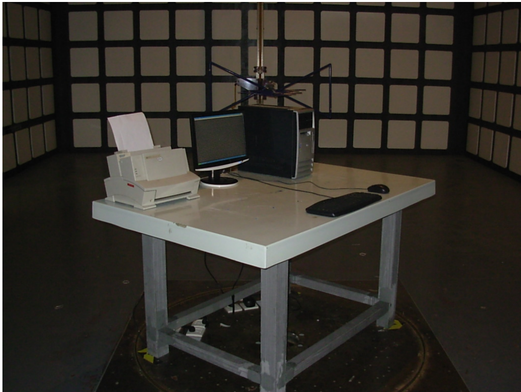
SETUP WITH MAXIMUM DETECTED EMISSION AT HORIZONTAL POLARIZATION (VGA 1440*900@60Hz, BELOW 1GHz)
