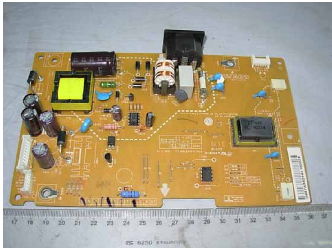
FIGURE 3 LCD MONITOR (M/N: W1946PW) POWER BOARD (COMPONENT SIDE)
