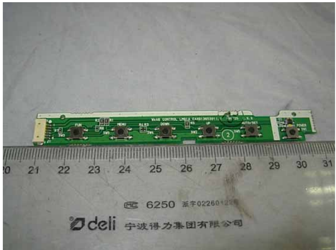
FIGURE 10 LCD MONITOR (M/N: W1946PW) KEY BOARD (COMPONENT SIDE)
