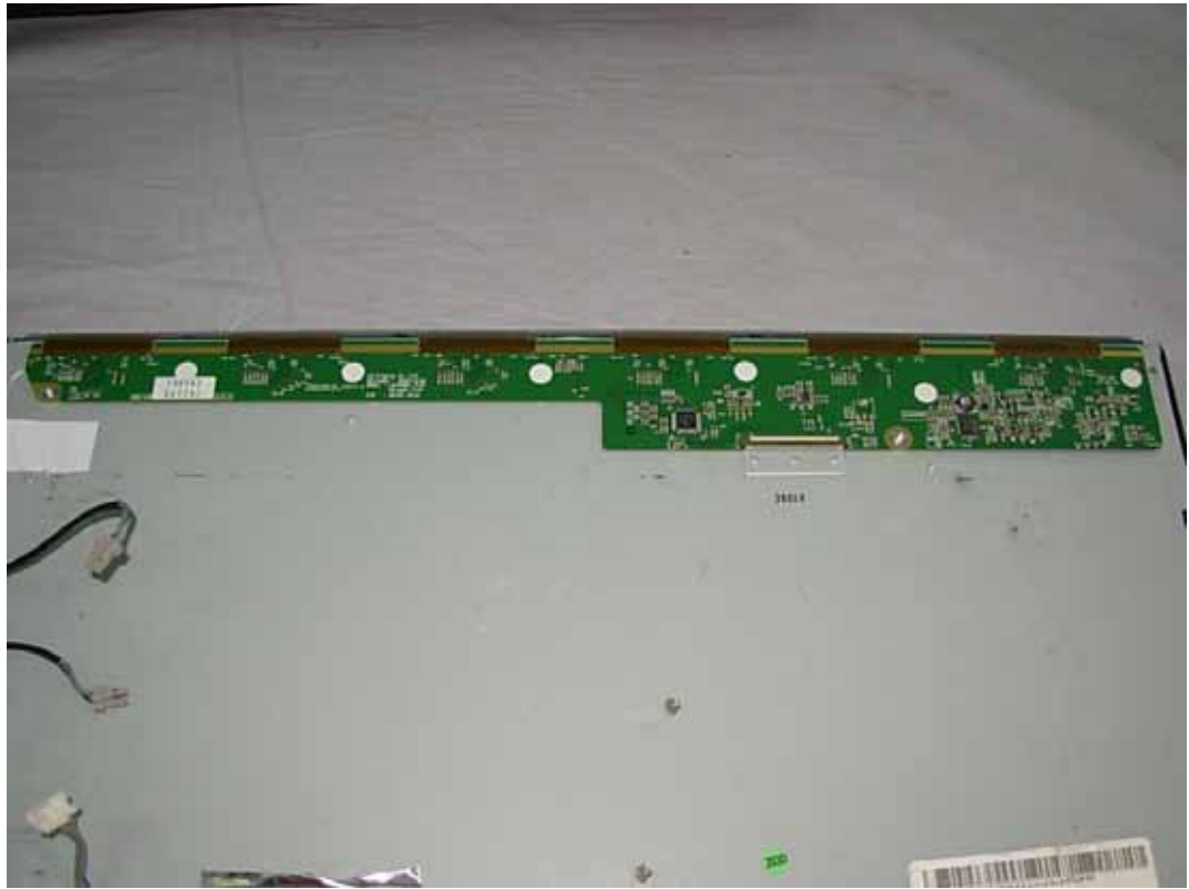
FIGURE 8 LCD MONITOR (M/N: W1946PW) DISPLAY BOARD (COMPONENT SIDE)
