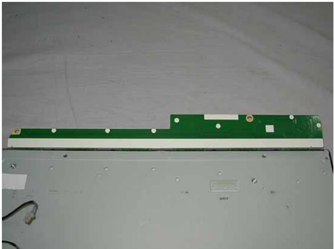
FIGURE 9 LCD MONITOR (M/N: W1946PW) DISPLAY BOARD (SOLDERED SIDE)
