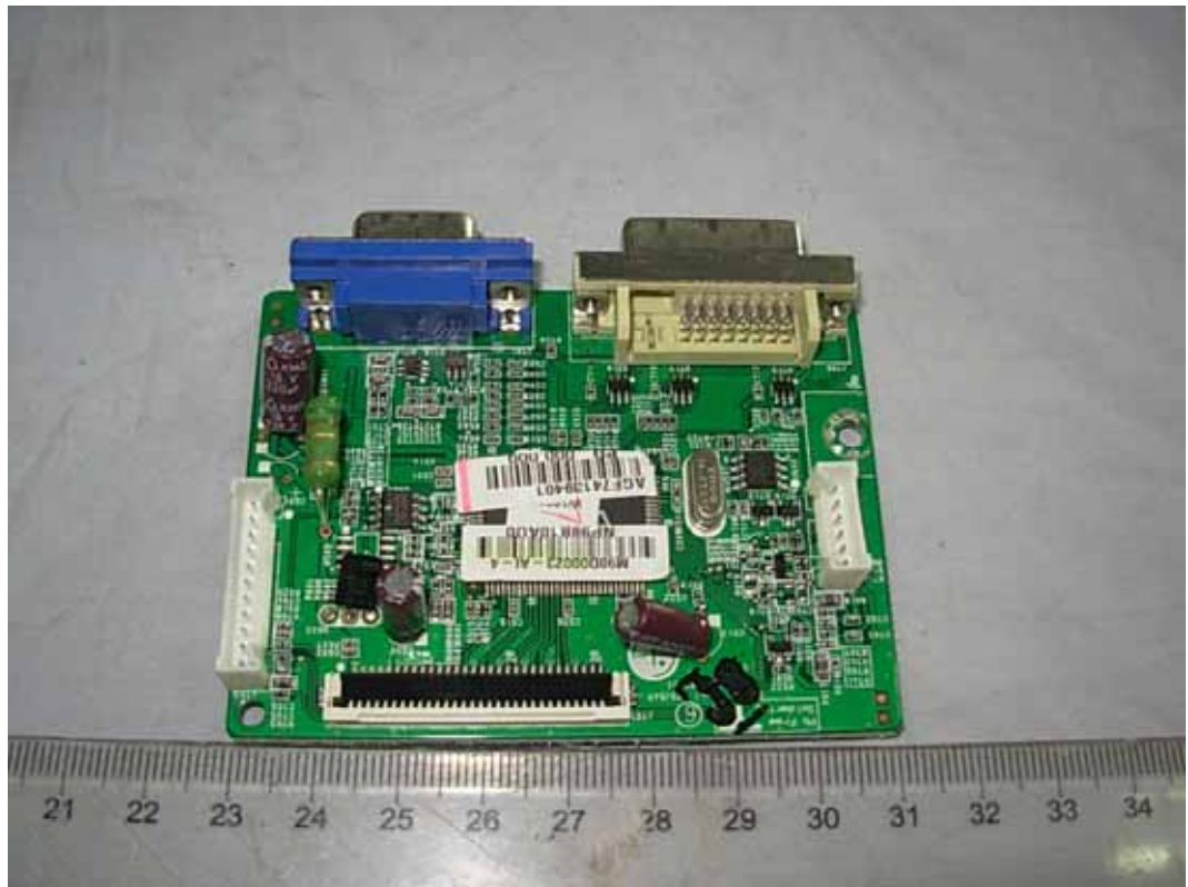
FIGURE 5 LCD MONITOR (M/N: W1946PW) MAIN BOARD (COMPONENT SIDE)
