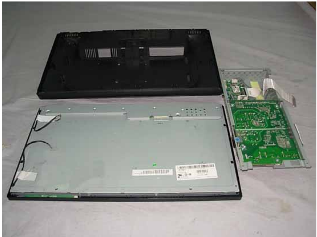
FIGURE 1 LCD MONITOR (M/N: W1946PW) COVER REMOVED
