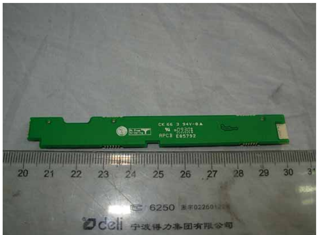
FIGURE 11 LCD MONITOR (M/N: W1946PW) KEY BOARD (SOLDERED SIDE)
