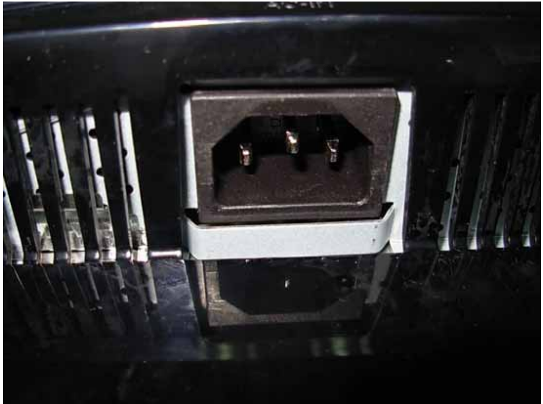
FIGURE 5 LCD MONITOR (M/N: W2040SV) POWER PORT
