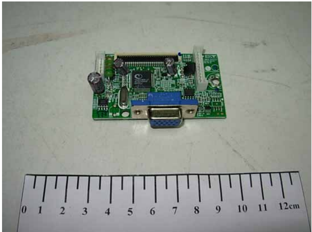
FIGURE 5 LCD MONITOR (M/N: W2040SV) MAIN BOARD (COMPONENT SIDE)
