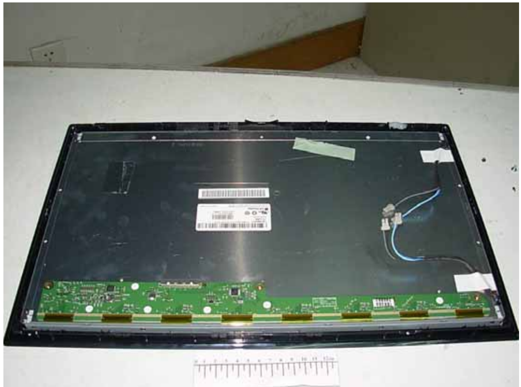
FIGURE 11 LCD MONITOR (M/N: W2040SV) LCD PANEL MAIN BOARD (COMPONENT SIDE)
