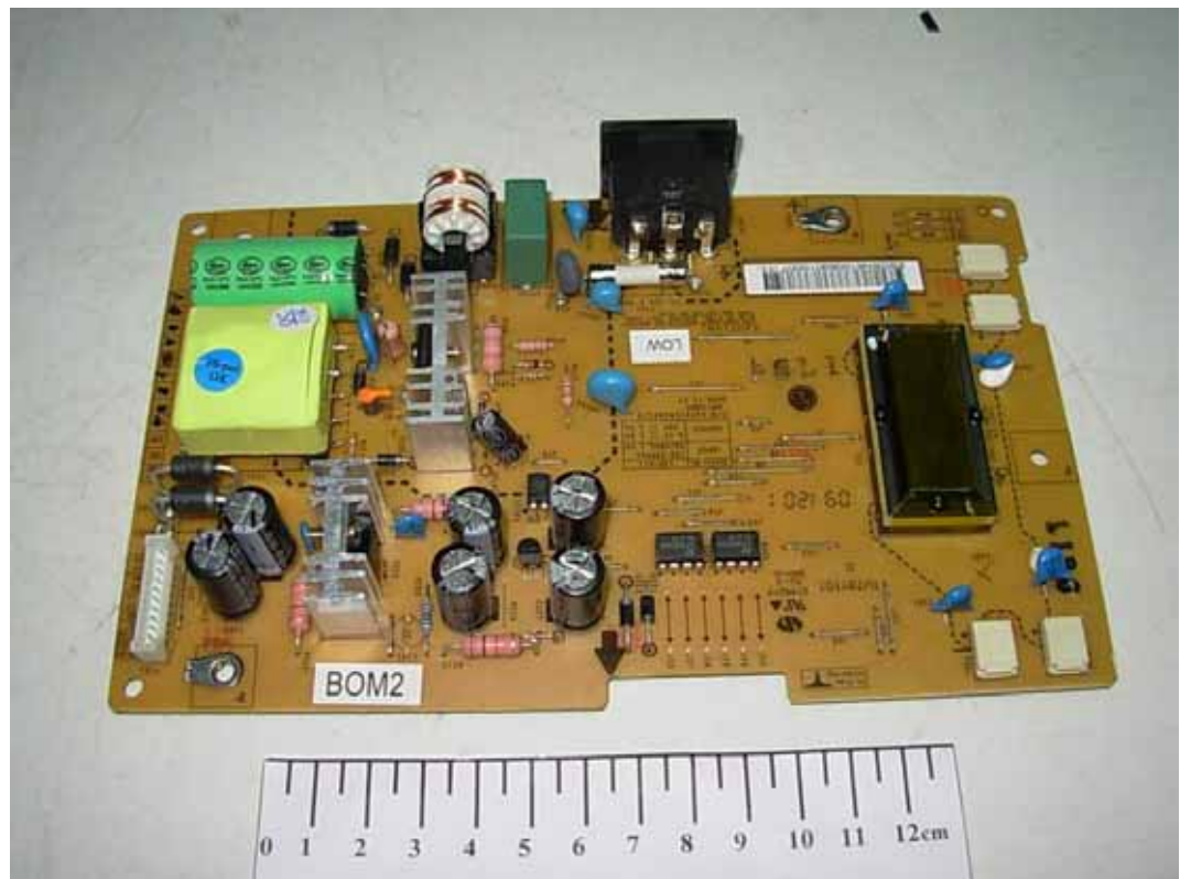
FIGURE 8 LCD MONITOR (M/N: W2040SV) POWER BOARD (COMPONENT SIDE)
