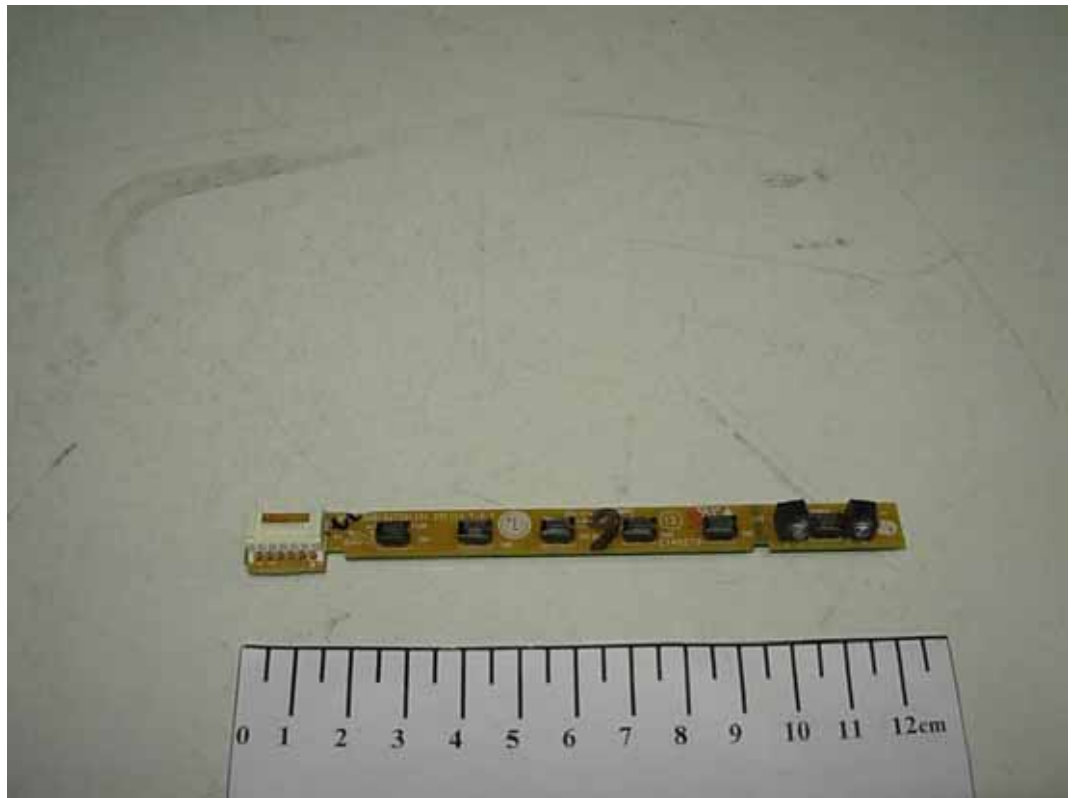
FIGURE 3 LCD MONITOR (M/N: W2040SV) KEY BOARD (COMPONENT SIDE)
