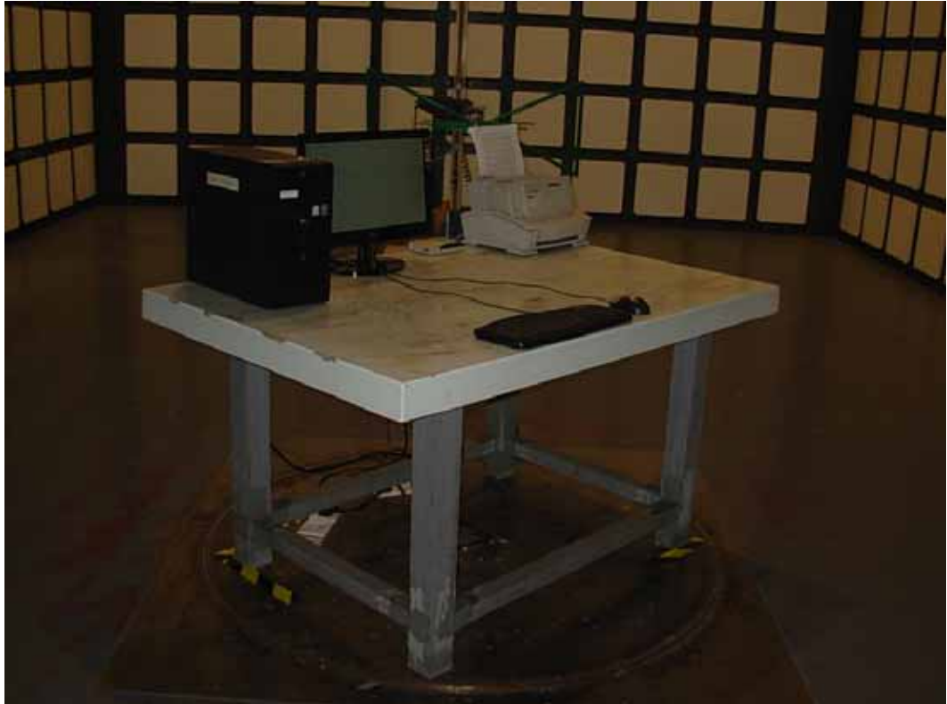
SETUP WITH MAXIMUM DETECTED EMISSION AT HORIZONTAL POLARIZATION (D-SUB 1600*900@60Hz)
