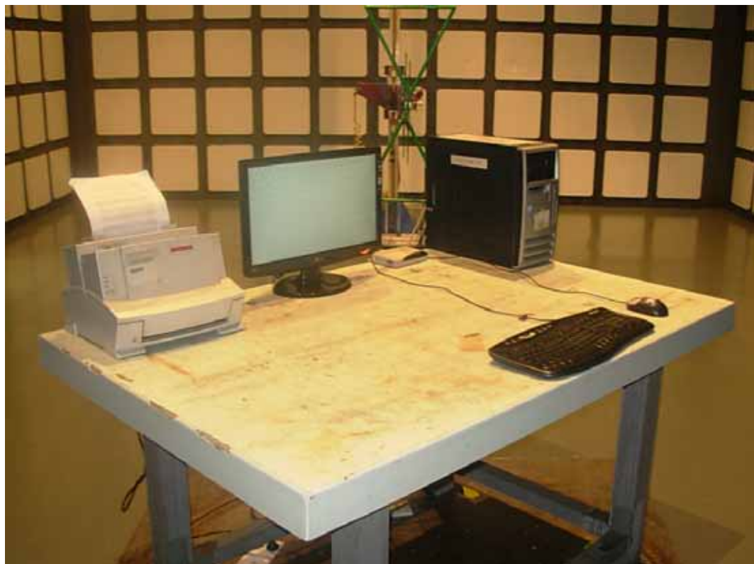
SETUP WITH MAXIMUM DETECTED EMISSION AT VERTICAL POLARIZATION (TEST MODE: D-SUB 1600*900@60Hz)
