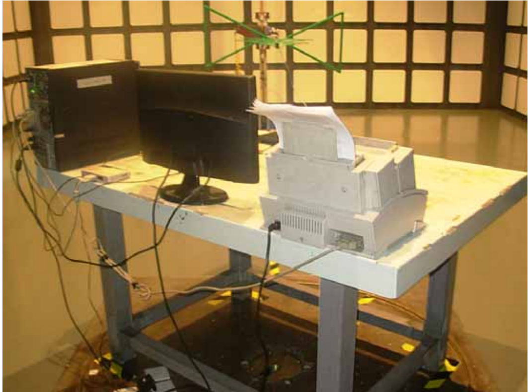
SETUP WITH MAXIMUM DETECTED EMISSION AT HORIZONTAL POLARIZATION (TEST MODE: D-SUB 1600*900@60Hz)
