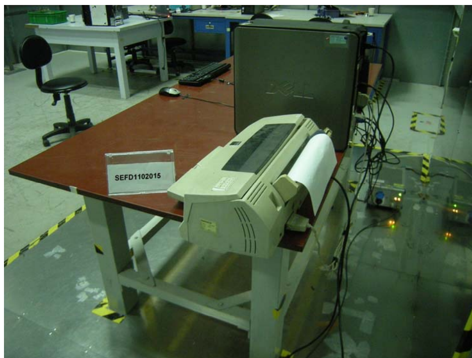
Back View of Conducted Emission Test
