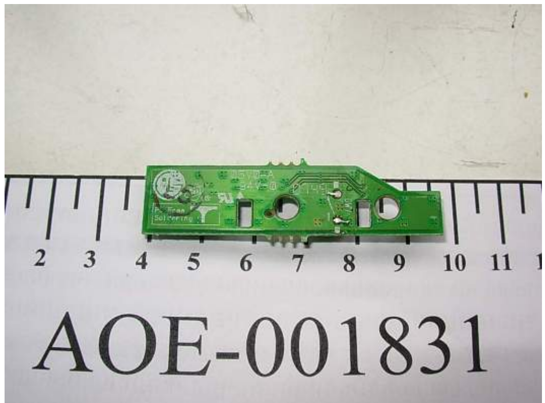
FIGURE 20 LCD MONITOR (M/N: W2052VQT) LED BOARD (SOLDERED SIDE)
