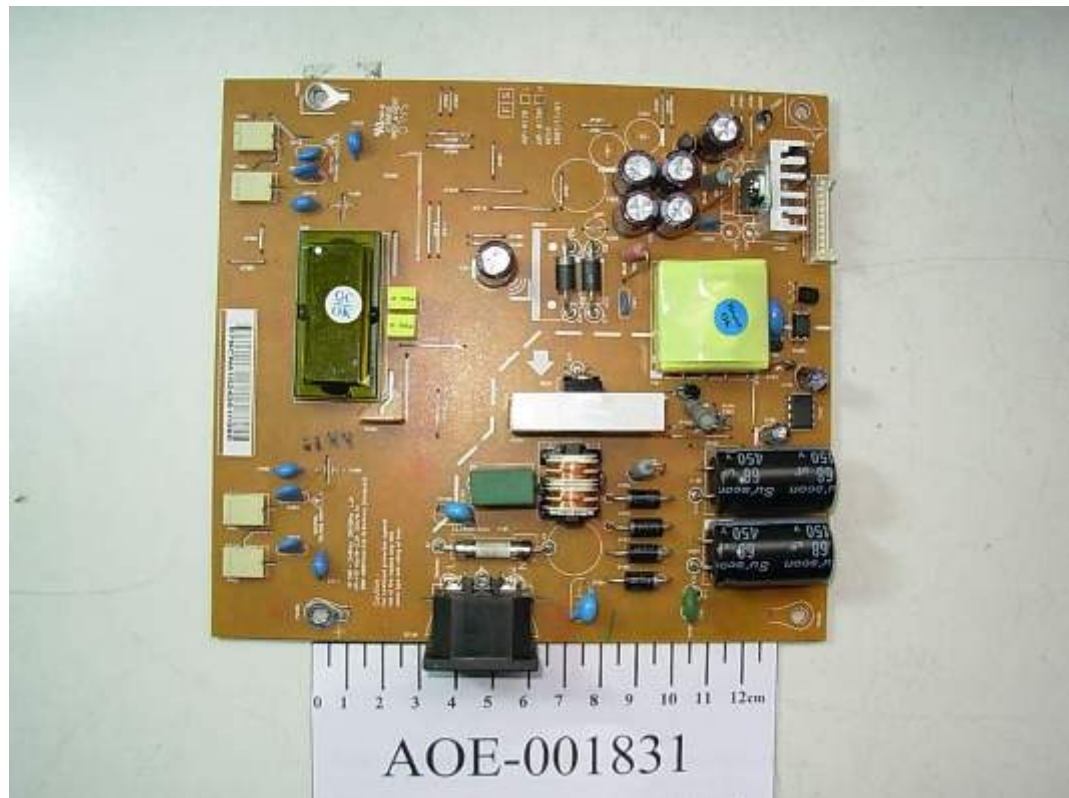
FIGURE 7 LCD MONITOR (M/N: W2052VQT) POWER BOARD (COMPONENT SIDE)
