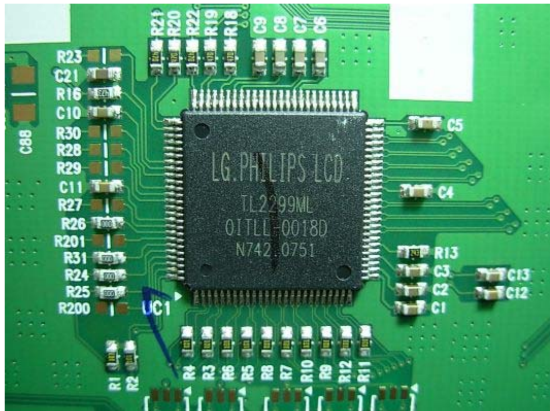
FIGURE 14 LCD MONITOR (M/N: W2052VQT) CHIP ON LCD PANEL MAIN BOARD
