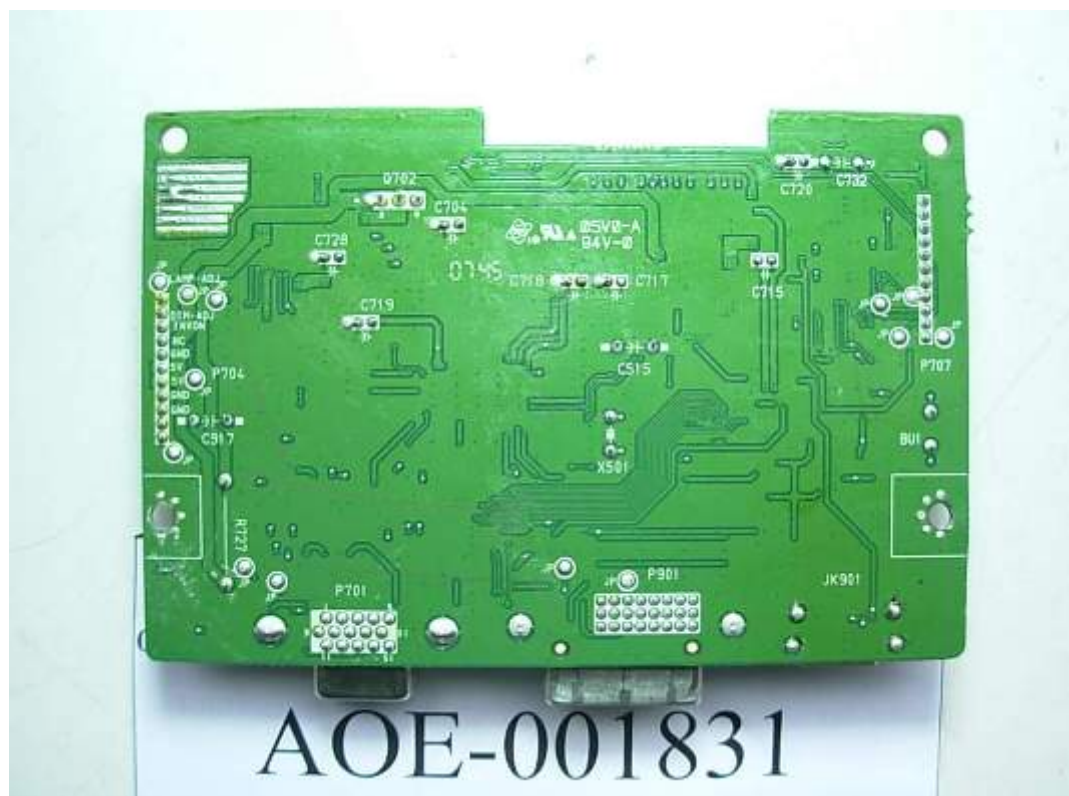
FIGURE 4 LCD MONITOR (M/N: W2052VQT) MAIN BOARD (SOLDERED SIDE)
