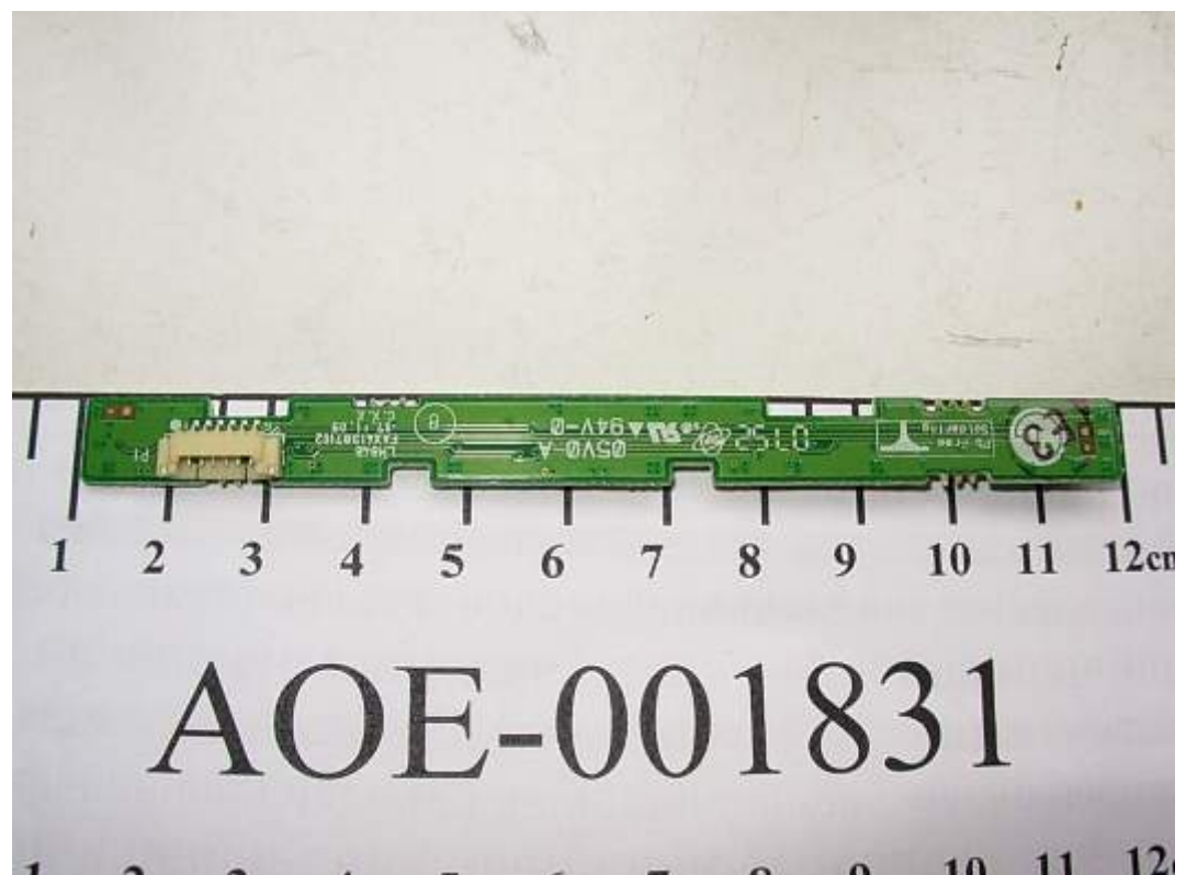
FIGURE 18 LCD MONITOR (M/N: W2052VQT) BUTTON BOARD (SOLDERED SIDE)
