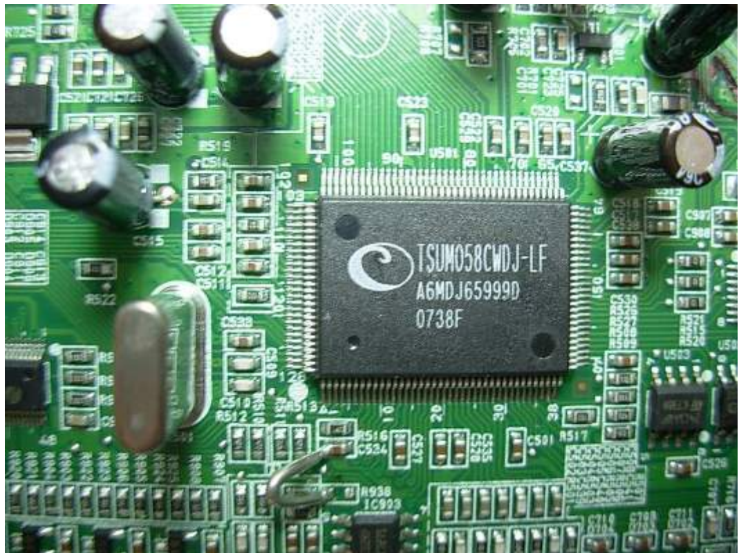
FIGURE 5 LCD MONITOR (M/N: W2052VQT) CHIP ON MAIN BOARD
