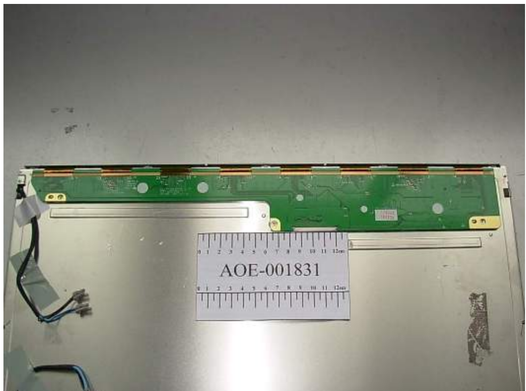
FIGURE 13 LCD MONITOR (M/N: W2052VQT) LCD PANEL MAIN BOARD (SOLDERED SIDE)
