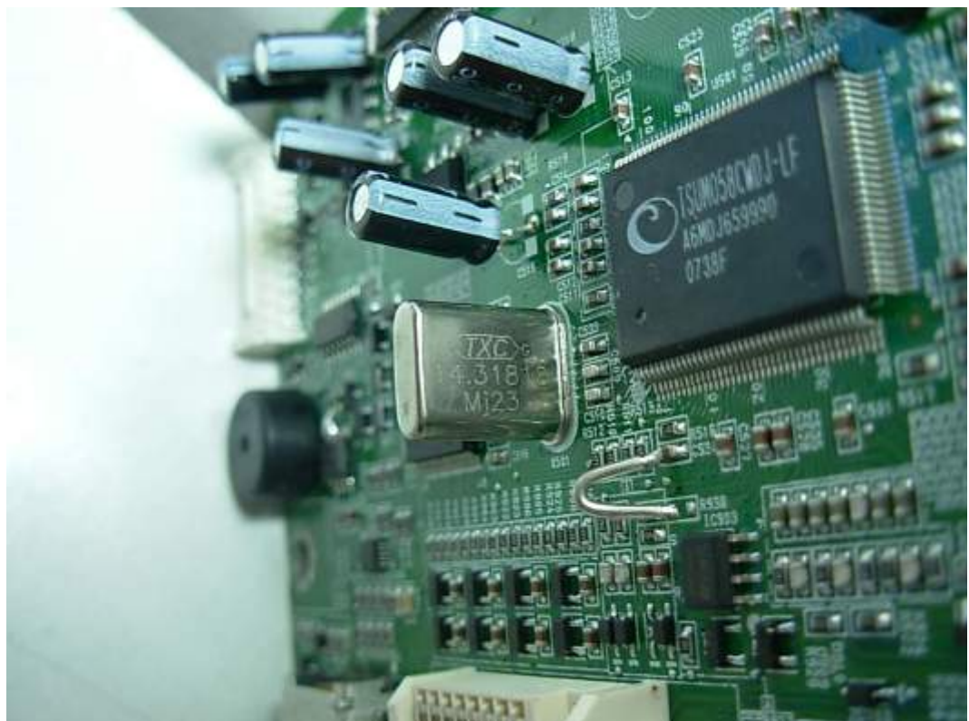
FIGURE 6 LCD MONITOR (M/N: W2052VQT) CRYSTAL ON MAIN BOARD
