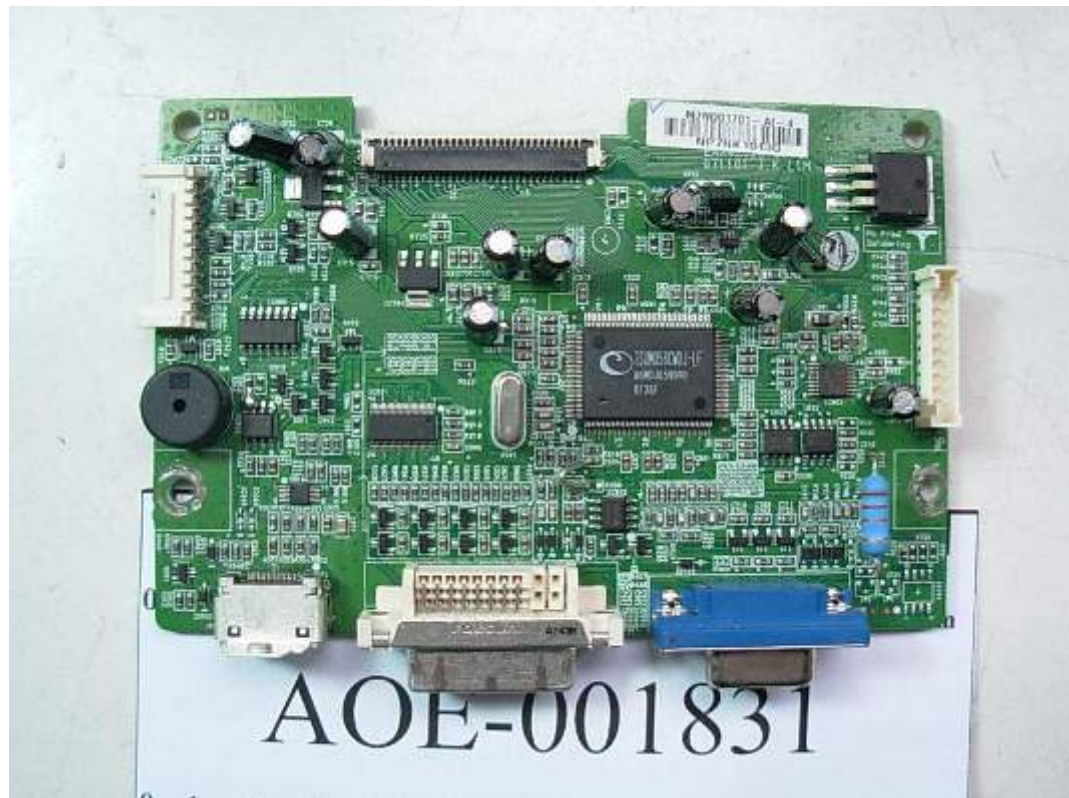
FIGURE 3 LCD MONITOR (M/N: W2052VQT) MAIN BOARD (COMPONENT SIDE)
