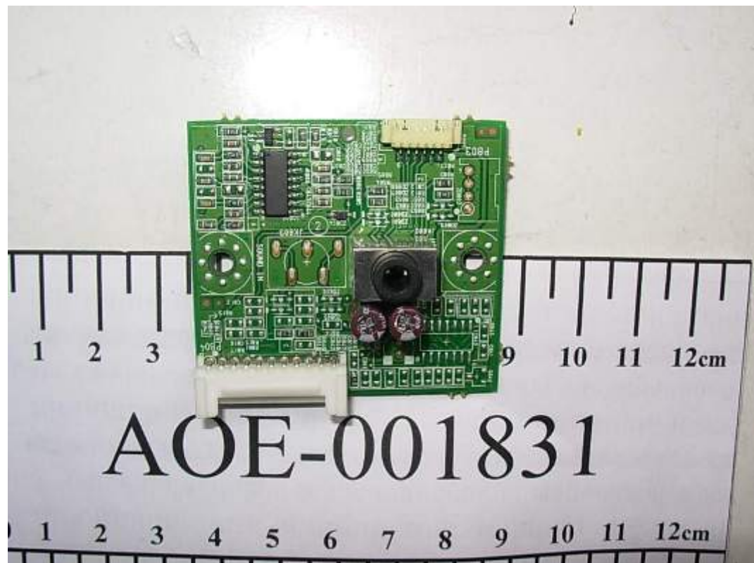
FIGURE 15 LCD MONITOR (M/N: W2052VQT) AUDIO BOARD (COMPONENT SIDE)
