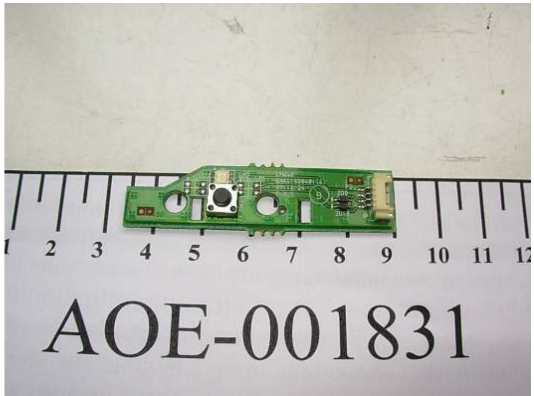
FIGURE 19 LCD MONITOR (M/N: W2052VQT) LED BOARD (COMPONENT SIDE)
