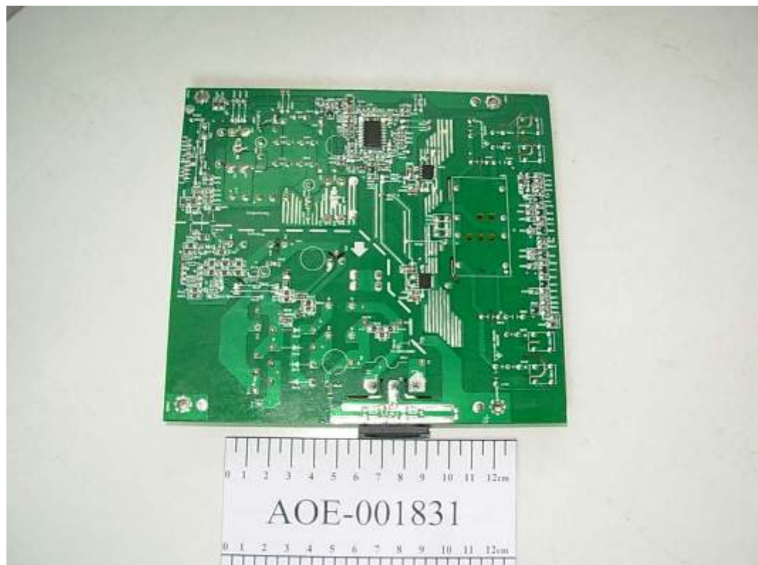
FIGURE 8 LCD MONITOR (M/N: W2052VQT) POWER BOARD (SOLDERED SIDE)
