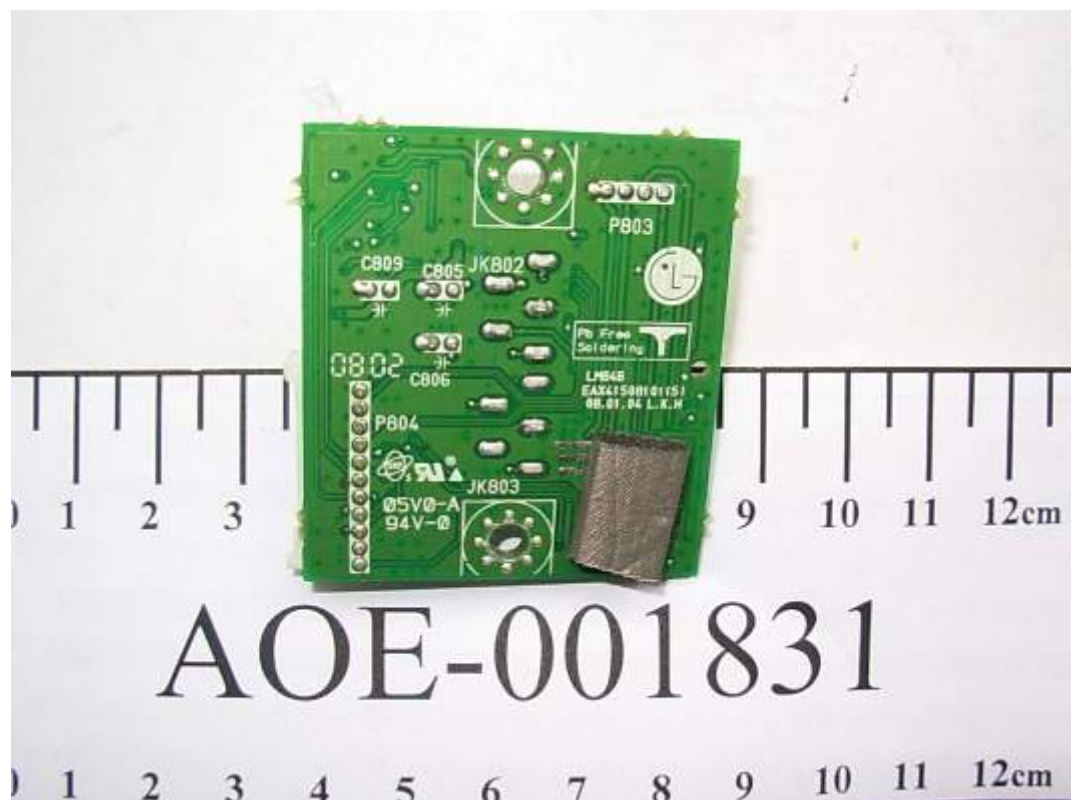
FIGURE 16 LCD MONITOR (M/N: W2052VQT) AUDIO BOARD (SOLDERED SIDE)
