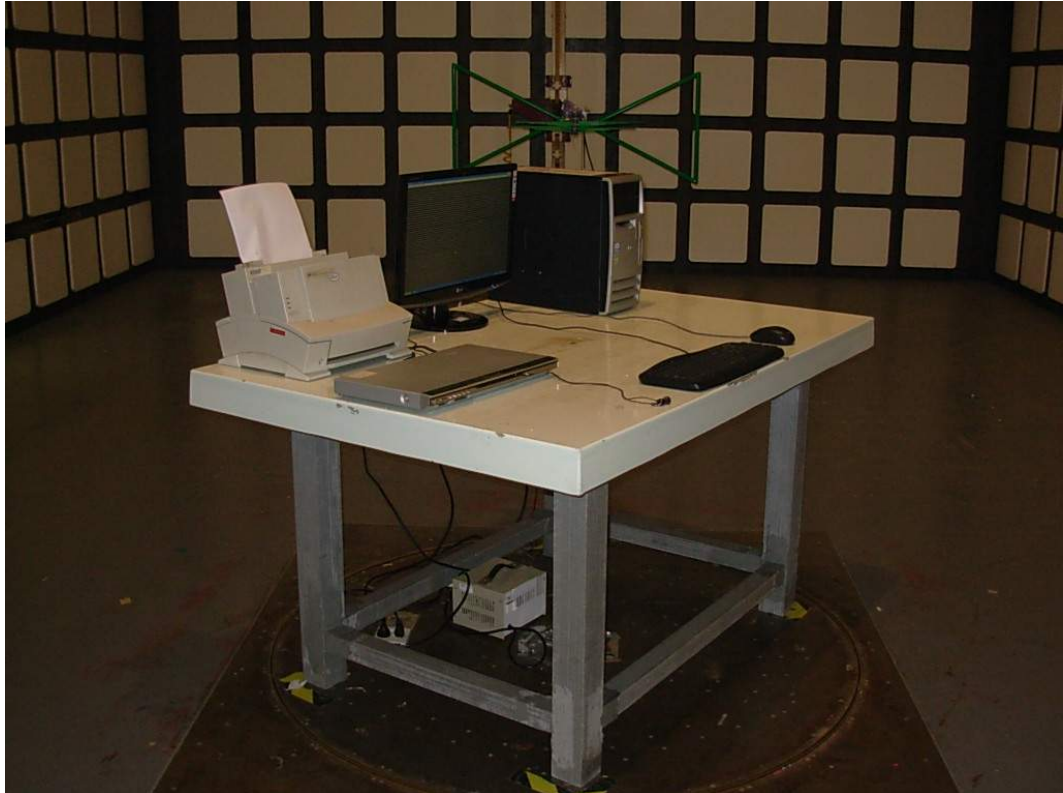
SETUP WITH MAXIMUM DETECTED EMISSION AT HORIZONTAL POLARIZATION (VGA 1680*1050@60Hz)
