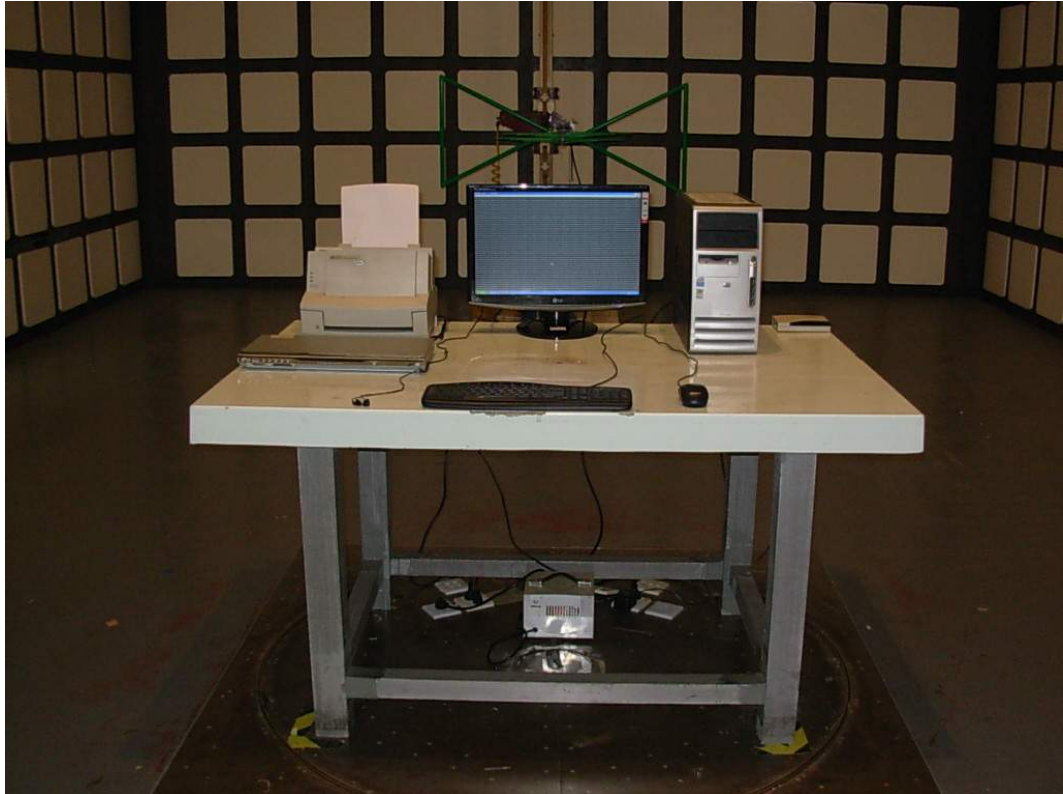
FRONT VIEW OF RADIATED EMISSION TEST
