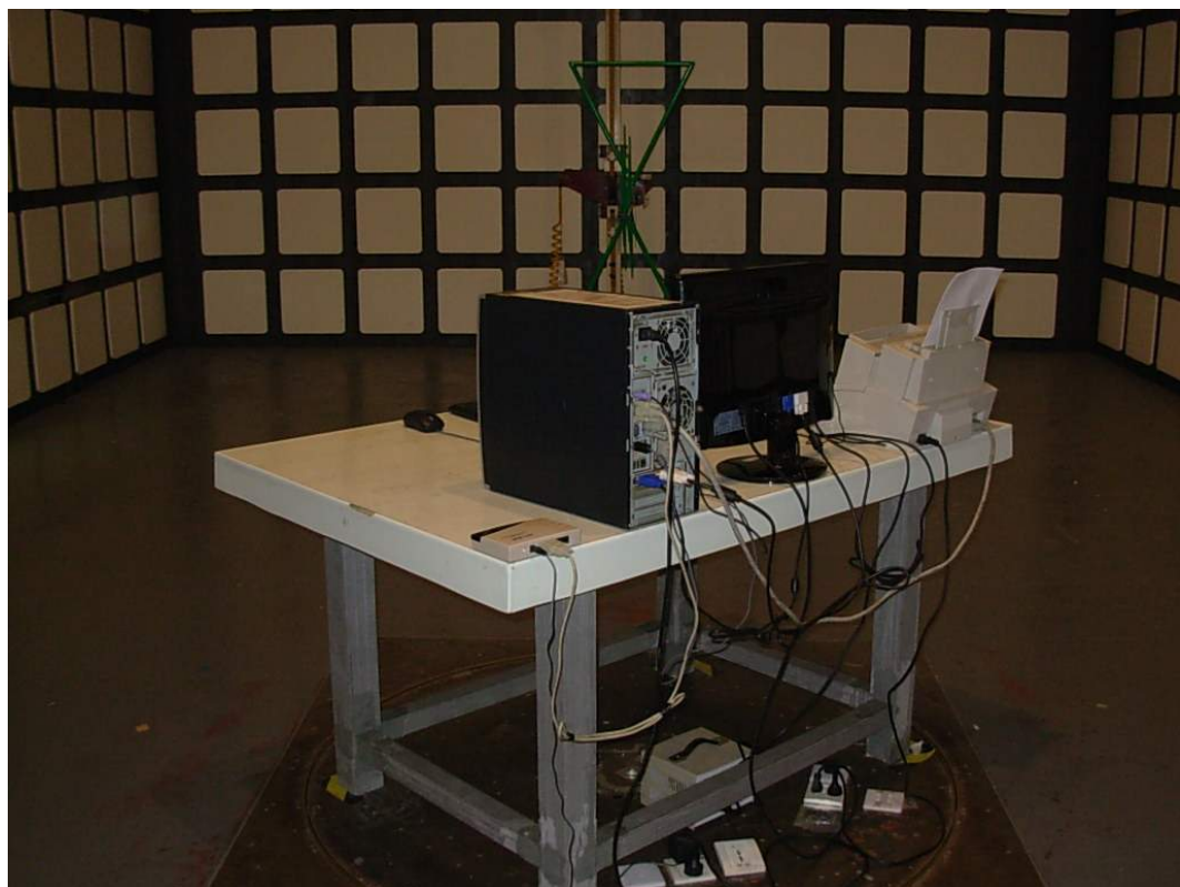
SETUP WITH MAXIMUM DETECTED EMISSION AT VERTICAL POLARIZATION (VGA 1680*1050@60Hz)
