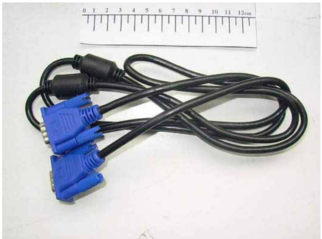
FIGURE 6 LCD MONITOR (M/N: W2240SV) D-SUB CABLE #1
