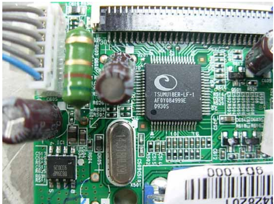
FIGURE 7 LCD MONITOR (M/N: W2240SV) CHIP & CRYSTAL ON MAIN BOARD
