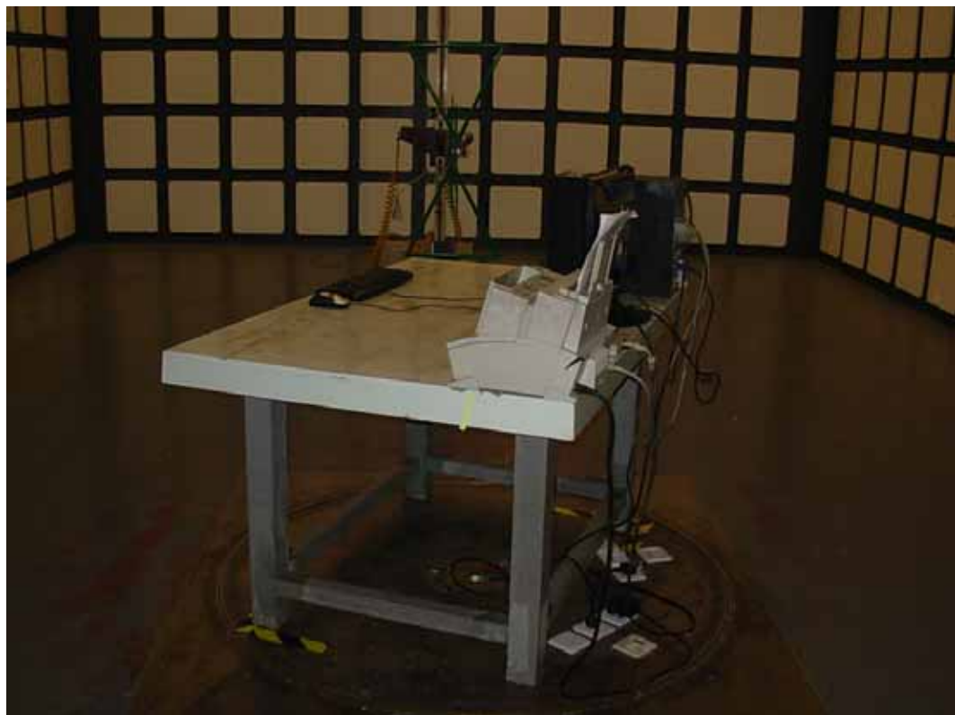
SETUP WITH MAXIMUM DETECTED EMISSION AT VERTICAL POLARIZATION (D-SUB 1680*1050@60Hz)
