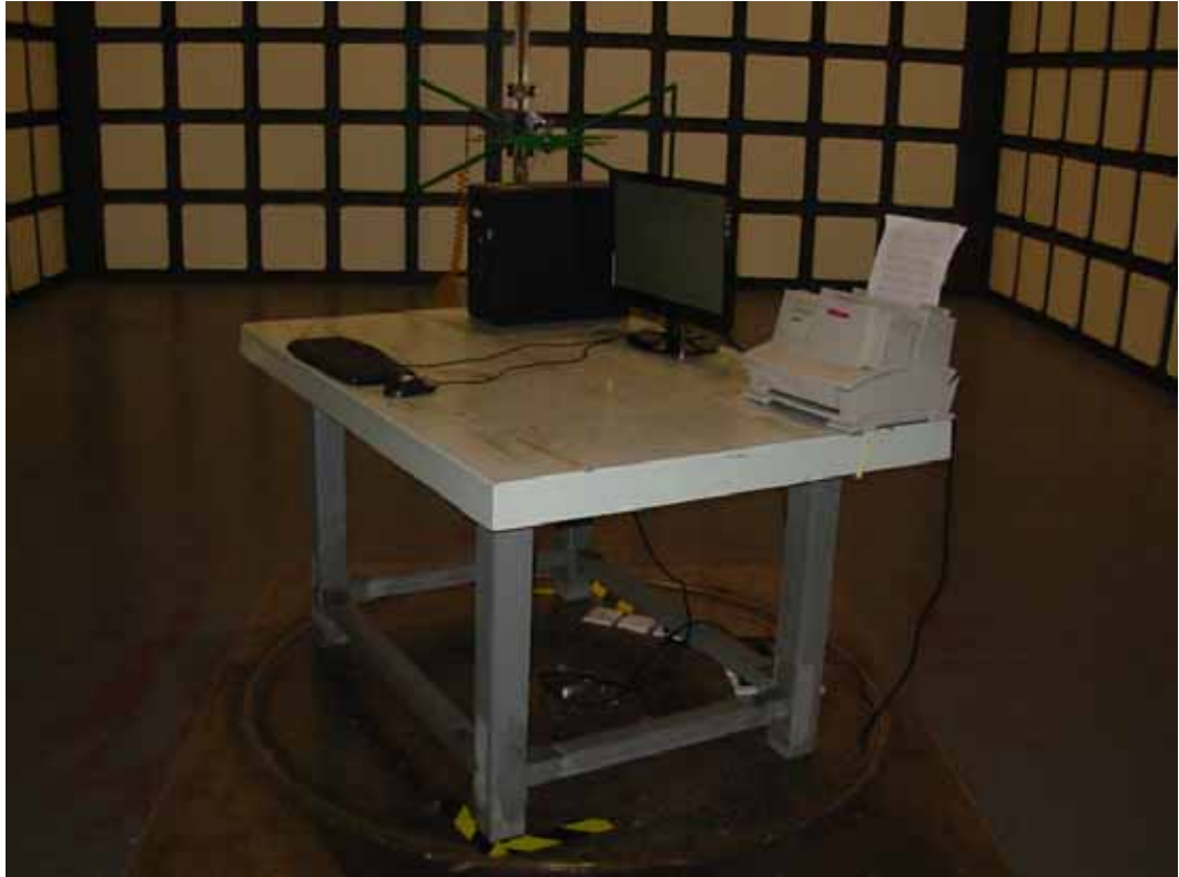
SETUP WITH MAXIMUM DETECTED EMISSION AT HORIZONTAL POLARIZATION (D-SUB 1680*1050@60Hz)
