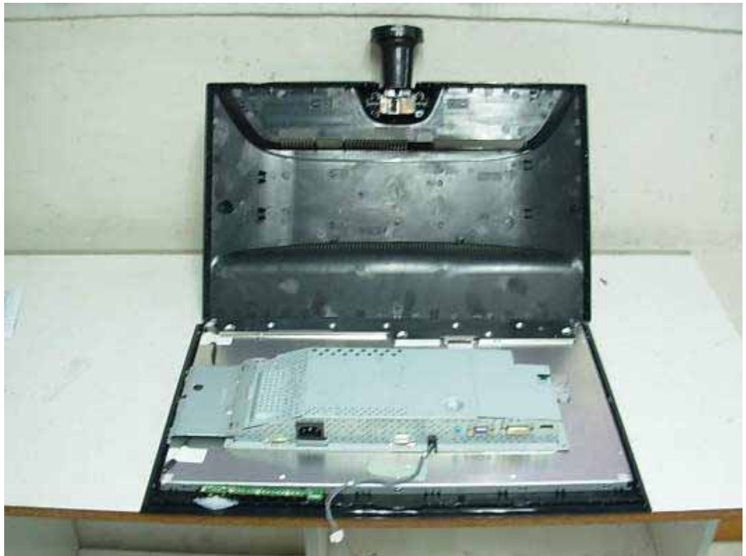
FIGURE 1 LCD MONITOR (M/N: W2240VV) COVER REMOVED
