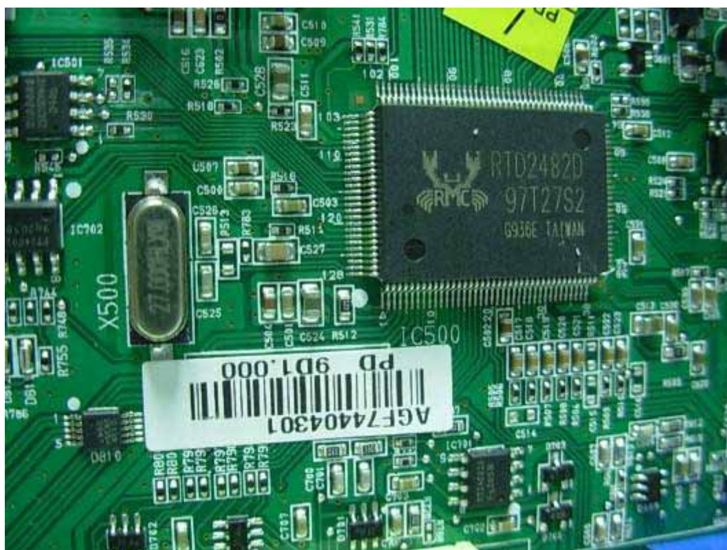
FIGURE 5 LCD MONITOR (M/N: W2240VV) CHIP & CRYSTAL ON MAIN BOARD
