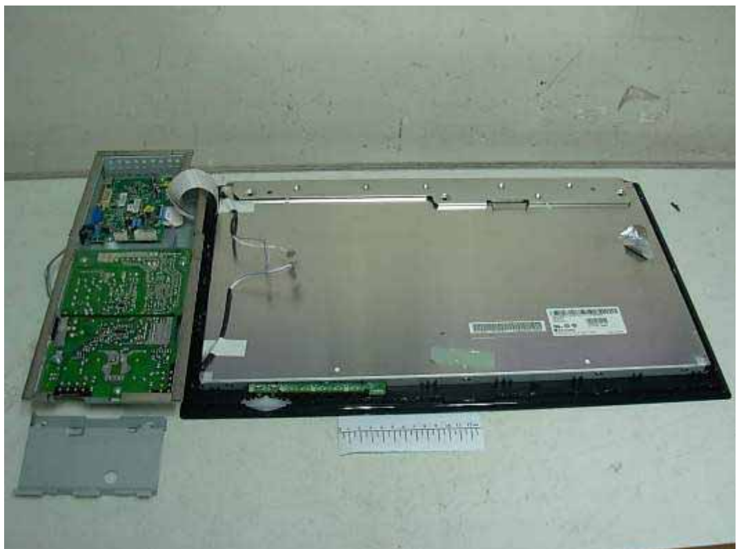
FIGURE 2 LCD MONITOR (M/N: W2240VV) BOARDS REMOVED
