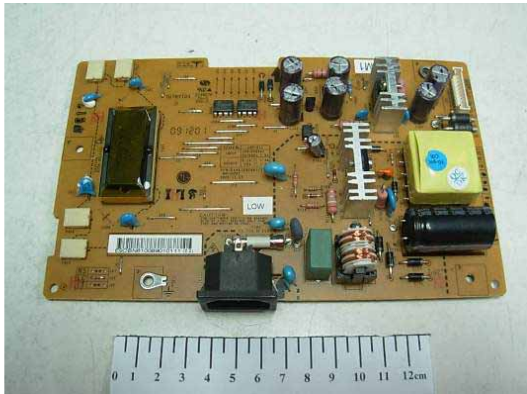
FIGURE 6 LCD MONITOR (M/N: W2240VV) POWER BOARD (COMPONENT SIDE)
