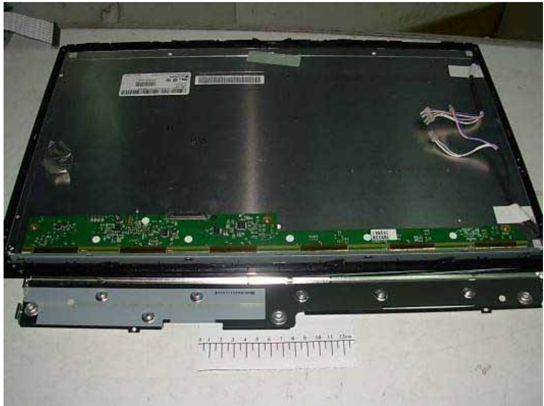
FIGURE 11 LCD MONITOR (M/N: W2240VV) LCD PANEL MAIN BOARD (COMPONENT SIDE)
