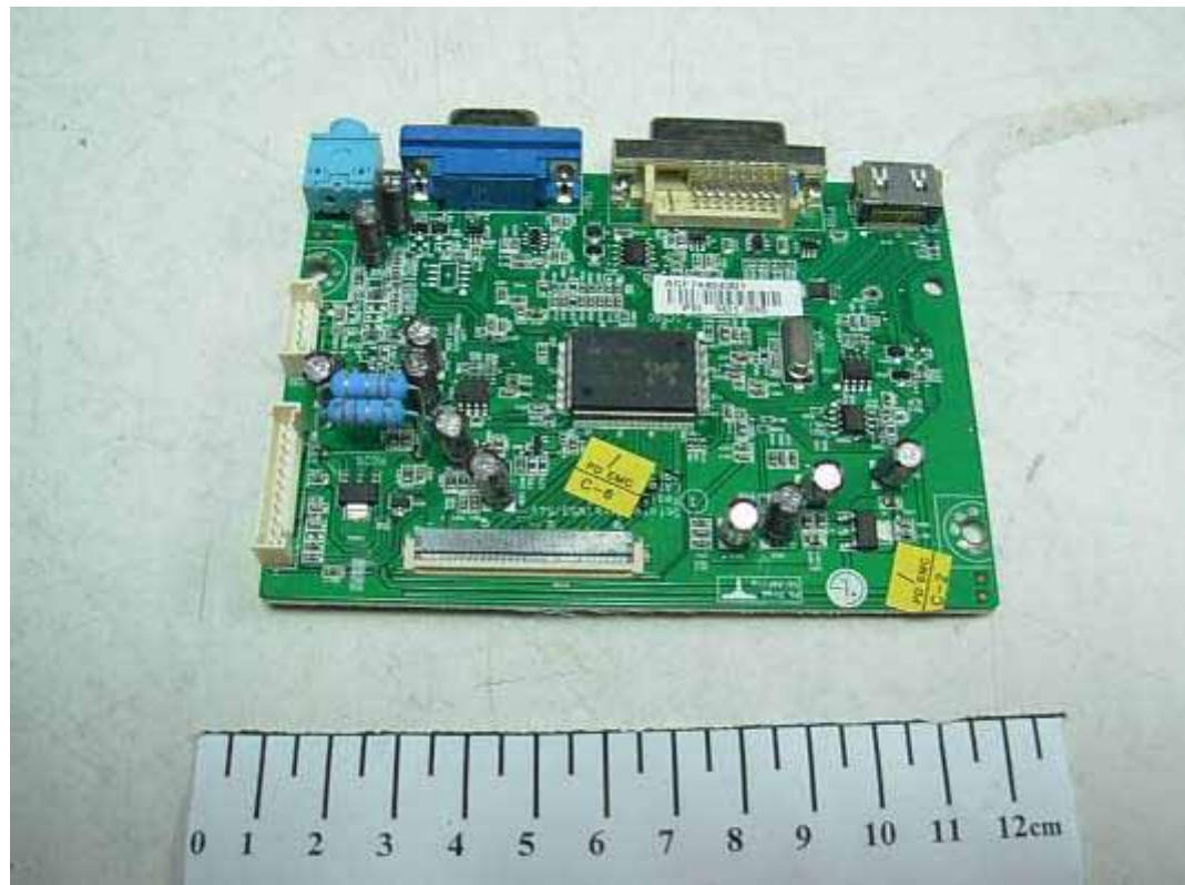
FIGURE 3 LCD MONITOR (M/N: W2240VV) MAIN BOARD (COMPONENT SIDE)
