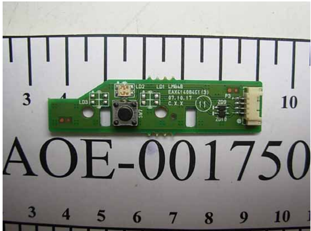
FIGURE 5 LCD MONITOR (M/N: W2252VQT) LED BOARD (COMPONENT SIDE)
