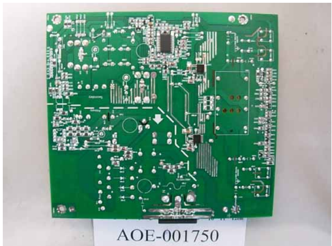
FIGURE 10 LCD MONITOR (M/N: W2252VQT) POWER BOARD (SOLDERED SIDE)
