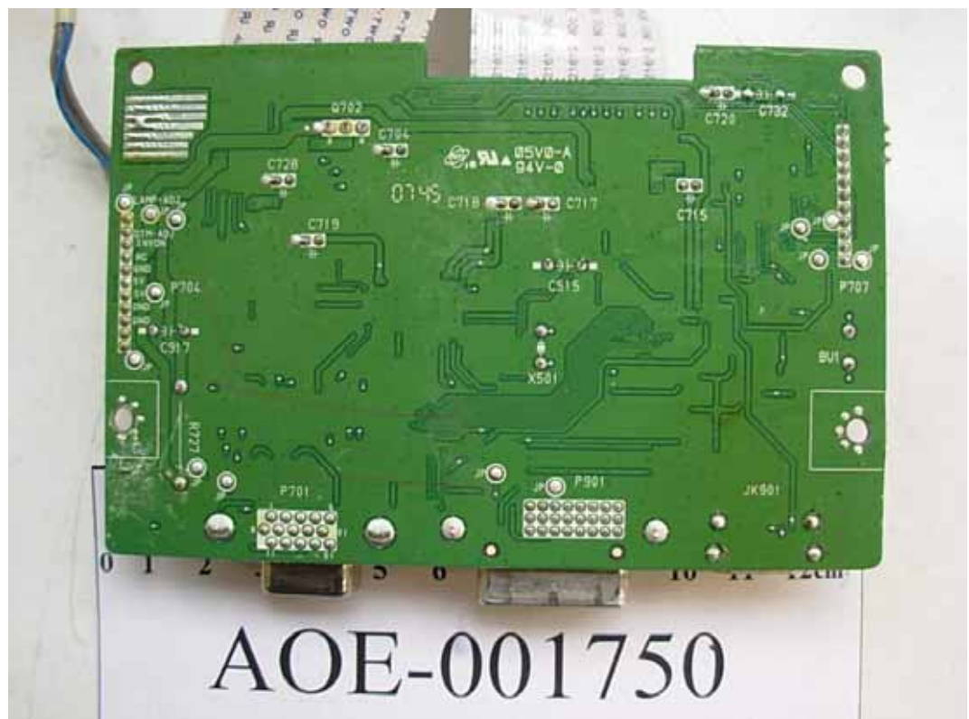
FIGURE 12 LCD MONITOR (M/N: W2252VQT) MAIN BOARD (SOLDERED SIDE)
