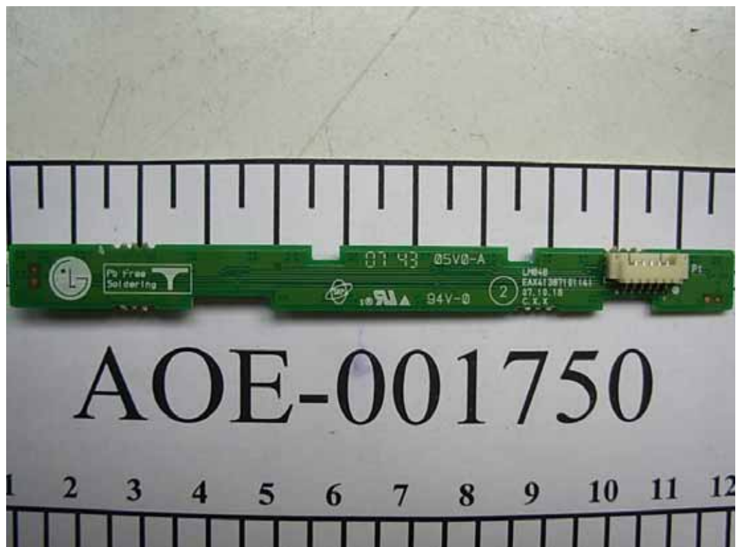
FIGURE 4 LCD MONITOR (M/N: W2252VQT) BUTTON BOARD (SOLDERED SIDE)
