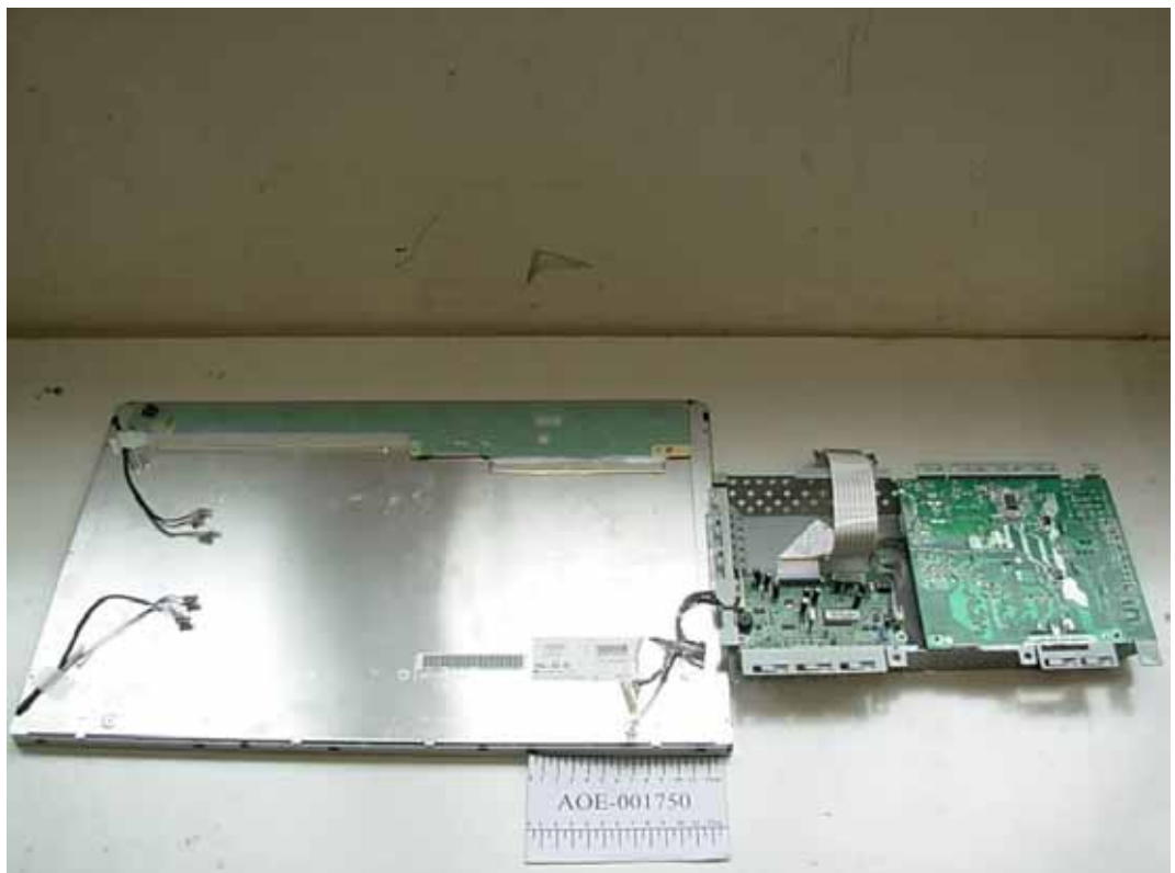
FIGURE 2 LCD MONITOR (M/N: W2252VQT) BOARDS REMOVED
