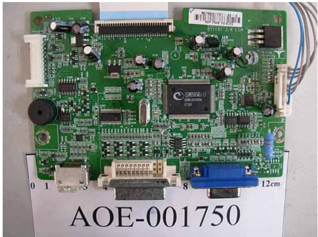
FIGURE 11 LCD MONITOR (M/N: W2252VQT) MAIN BOARD (COMPONENT SIDE)
