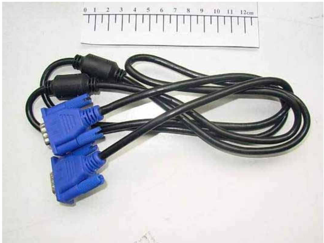
FIGURE 6 LCD MONITOR (M/N: W2340SV) D-SUB CABLE #1
