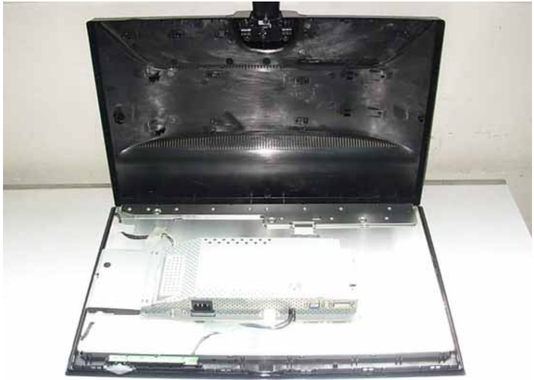
FIGURE 1 LCD MONITOR (M/N: W2340TV) COVER REMOVED
