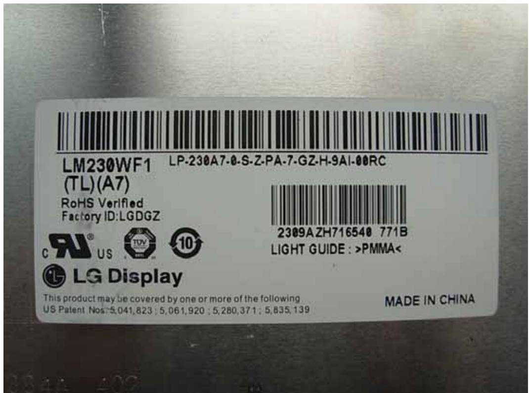
FIGURE 10 LCD MONITOR (M/N: W2340TV) LCD PANEL LABEL
