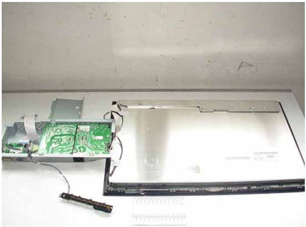
FIGURE 2 LCD MONITOR (M/N: W2340TV) BOARDS REMOVED
