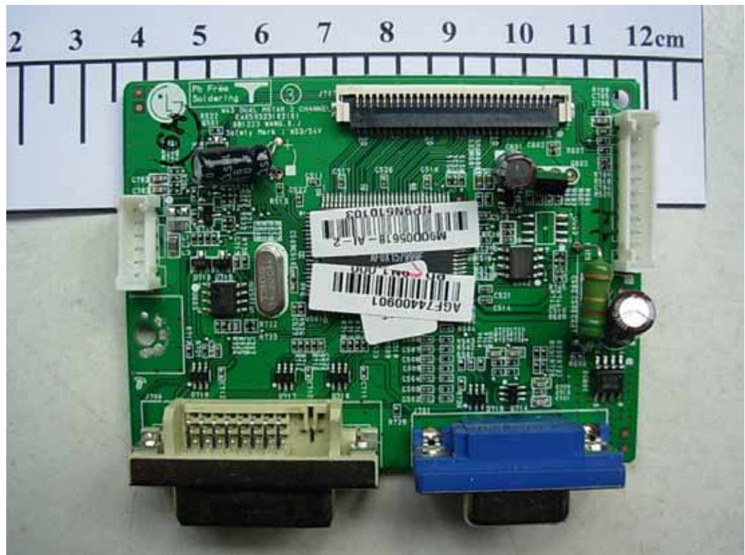
FIGURE 7 LCD MONITOR (M/N: W2340TV) MAIN BOARD (COMPONENT SIDE)
