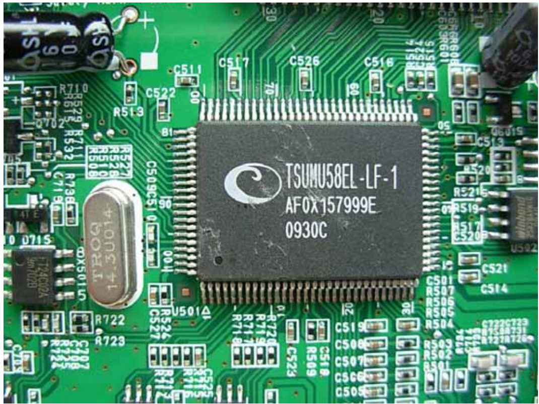
FIGURE 9 LCD MONITOR (M/N: W2340TV) CHIP & CRYSTAL ON MAIN BOARD
