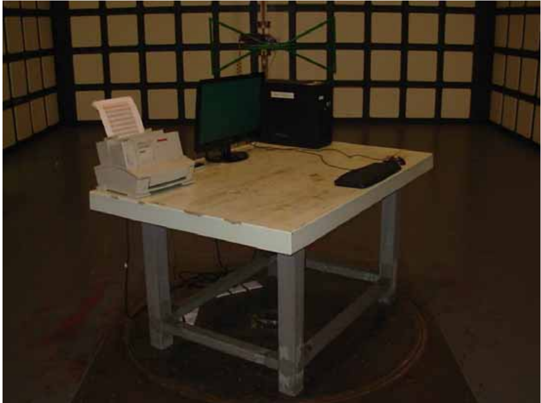
SETUP WITH MAXIMUM DETECTED EMISSION AT HORIZONTAL POLARIZATION (TEST MODE: DVI 640*480@60Hz)
