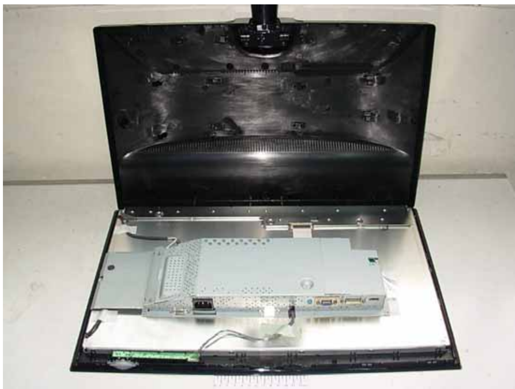
FIGURE 1 LCD MONITOR (M/N: W2340VV) COVER REMOVED
