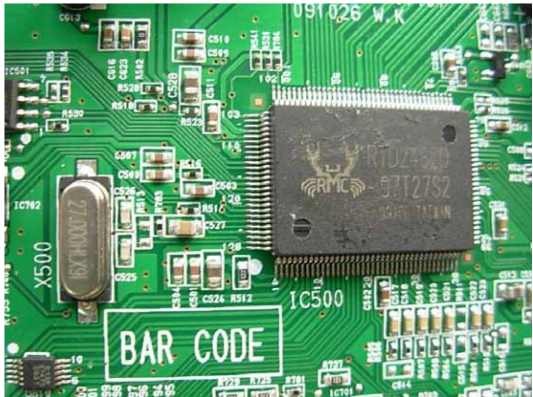
FIGURE 7 LCD MONITOR (M/N: W2340VV) CHIP & CRYSTAL ON MAIN BOARD
