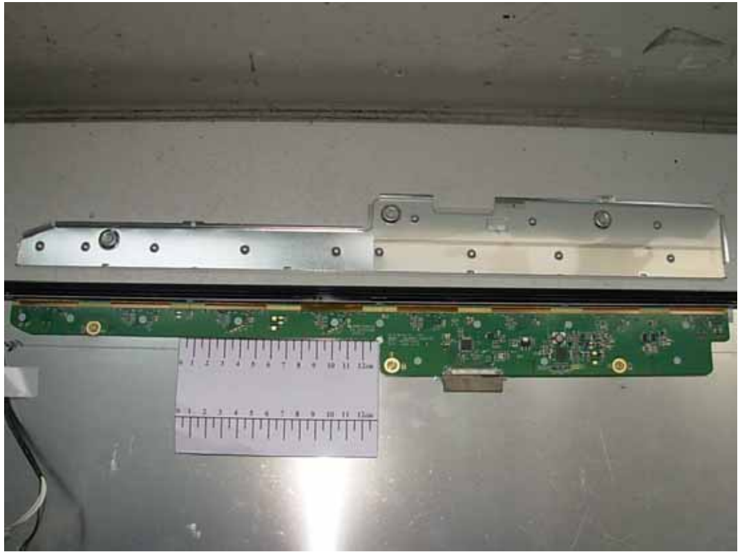
FIGURE 11 LCD MONITOR (M/N: W2340VV) LCD PANEL MAIN BOARD (COMPONENT SIDE)
