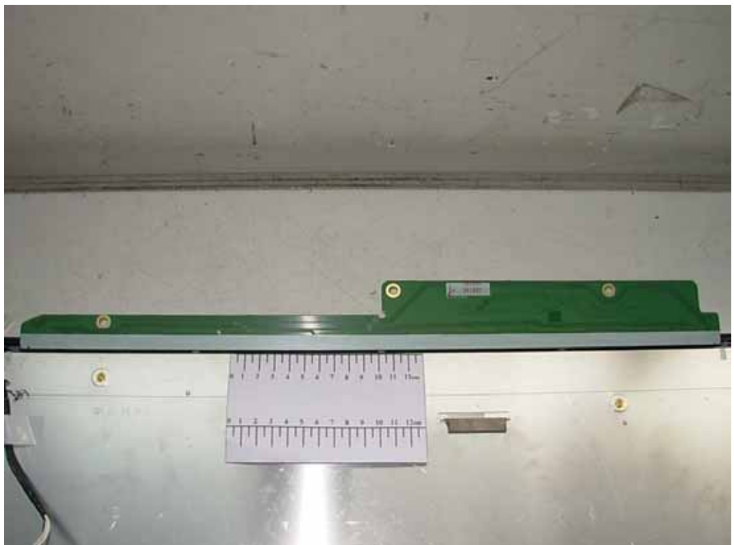
FIGURE 12 LCD MONITOR (M/N: W2340VV) LCD PANEL MAIN BOARD (SOLDERED SIDE)
