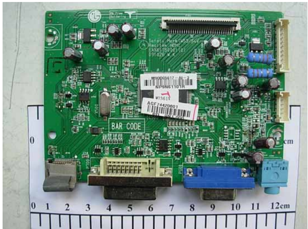
FIGURE 5 LCD MONITOR (M/N: E2350VV) MAIN BOARD (COMPONENT SIDE)
