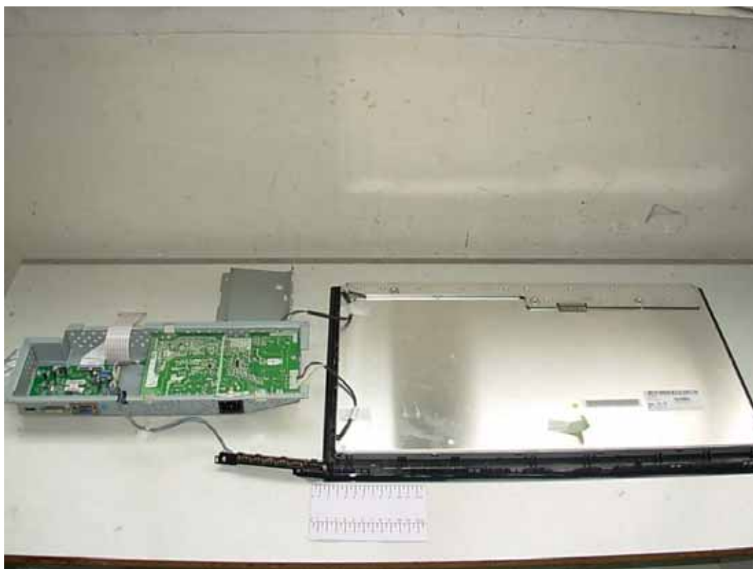
FIGURE 2 LCD MONITOR (M/N: W2340VV) BOARDS REMOVED
