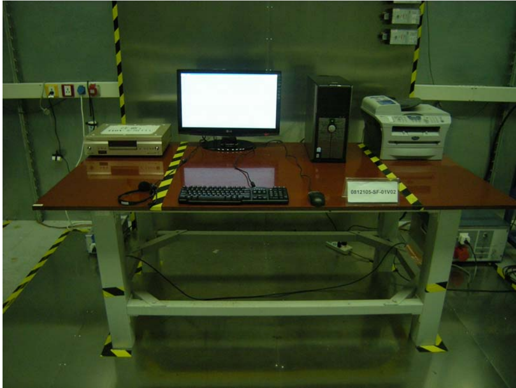
Front View of Conducted Emission Test
