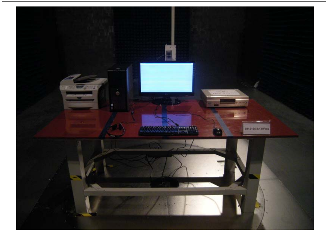
Front View of Radiated Emission Test (Above 1G)
