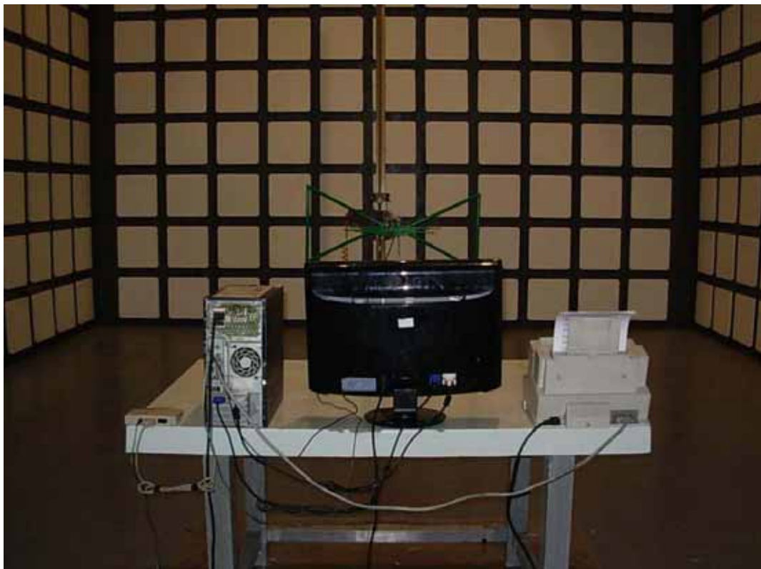
BACK VIEW OF RADIATED EMISSION TEST
