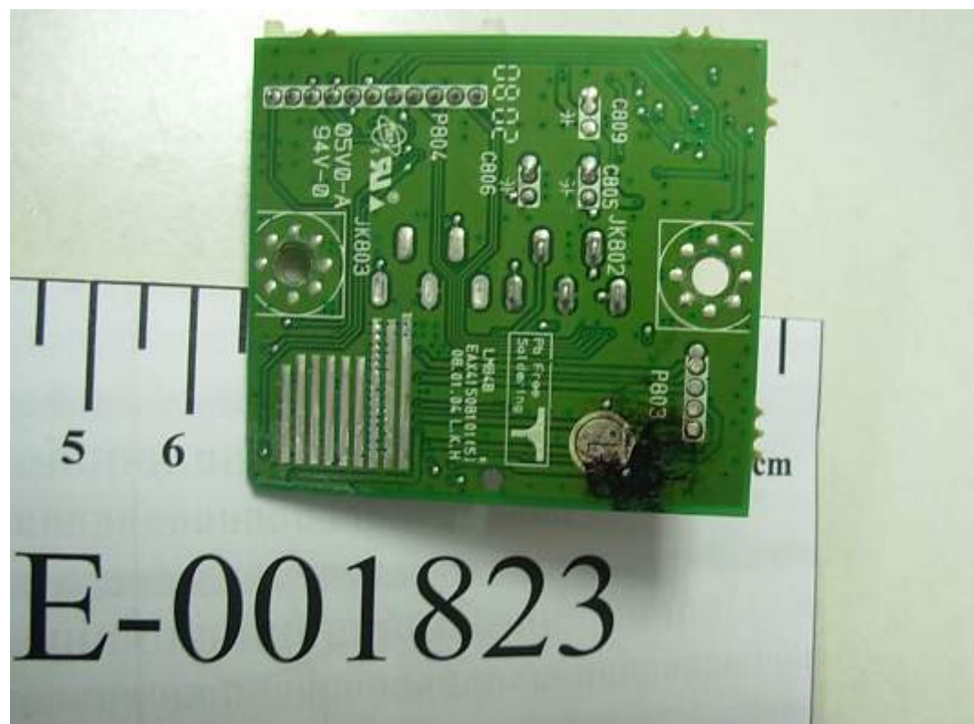
FIGURE 7 LCD MONITOR (M/N: W2452VQT) AUDIO BOARD (SOLDERED SIDE)
