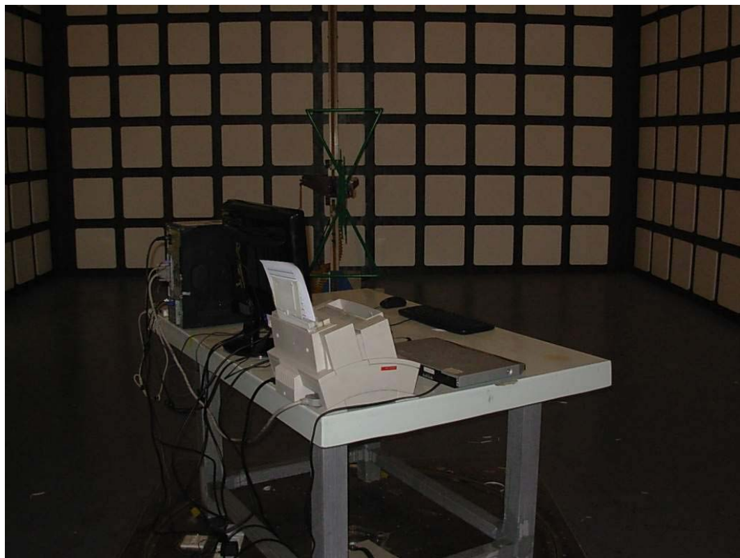
SETUP WITH MAXIMUM DETECTED EMISSION AT VERTICAL POLARIZATION (DVI 1680*1050@60Hz)
