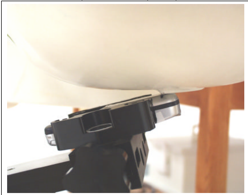
EUT Setup Configuration 1 (Left Head -Tilted position)
