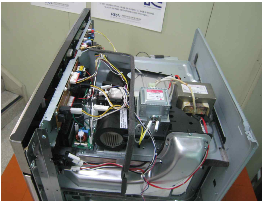
<Inside of MWO>
