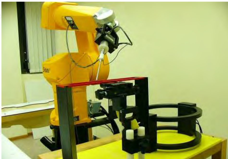
Fig.1 Photograph of the DASY 4 measurement System
