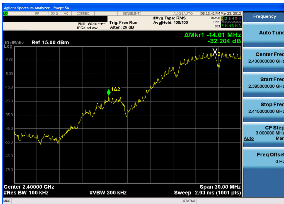
Plot 6-19. Band Edge Plot (802.11b – Ch. 1)
