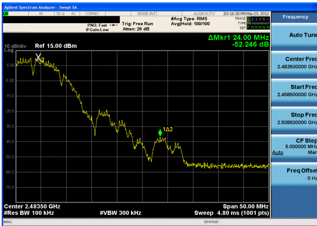
Plot 6-20. Band Edge Plot (802.11b - Ch. 11)
