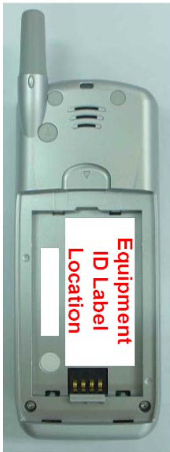
Rear View (with Battery Removed To Show Equipment ID Label)
