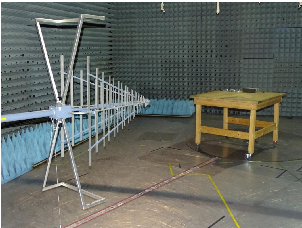
Photo 2: Test setup for radiated measurements (30 MHz - 1 GHz)
