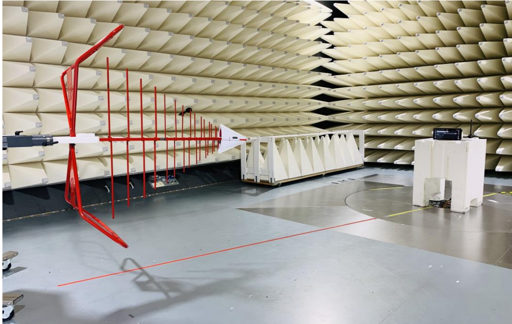
Figure C3. Radiated Setup – Low Range
