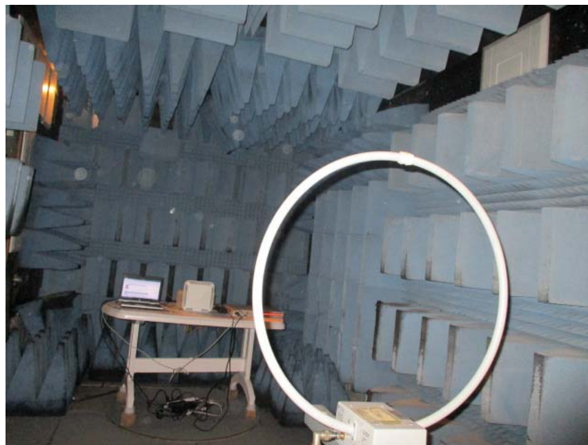
Figure 4. Radiated Emission Test, 0.009-30MHz
