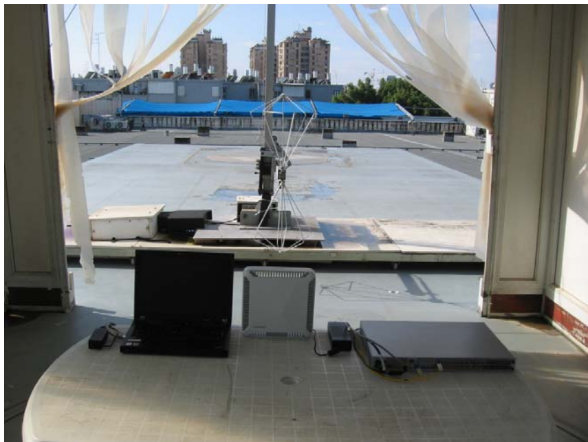
Figure 5. Radiated Emission Test, 30-200MHz
