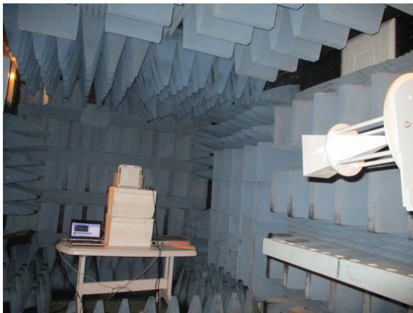
Figure 8. Radiated Emission Test, 18-26.5GHz
