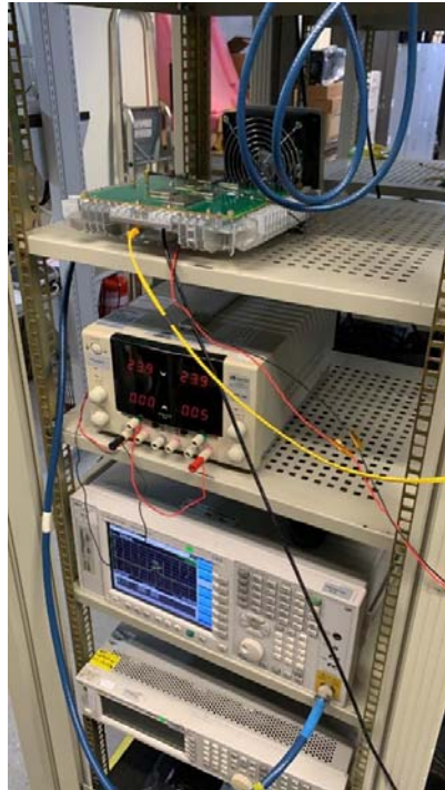
Figure 3. Conducted Test Set-Up
