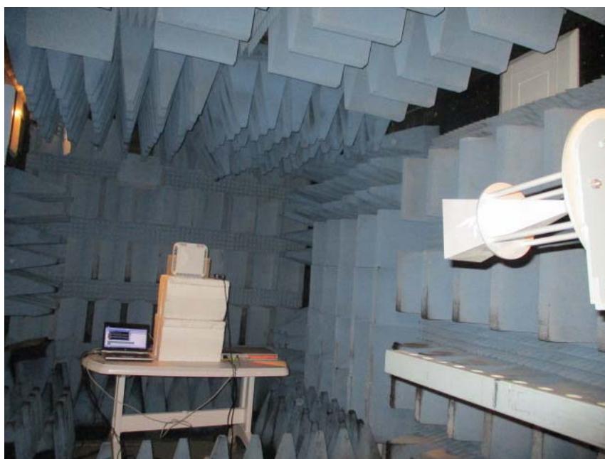
Figure 8. Radiated Emission Test, 18-26.5GHz
