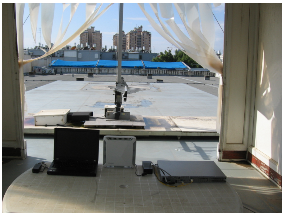
Radiated Emission Test, 200-1000MHz
